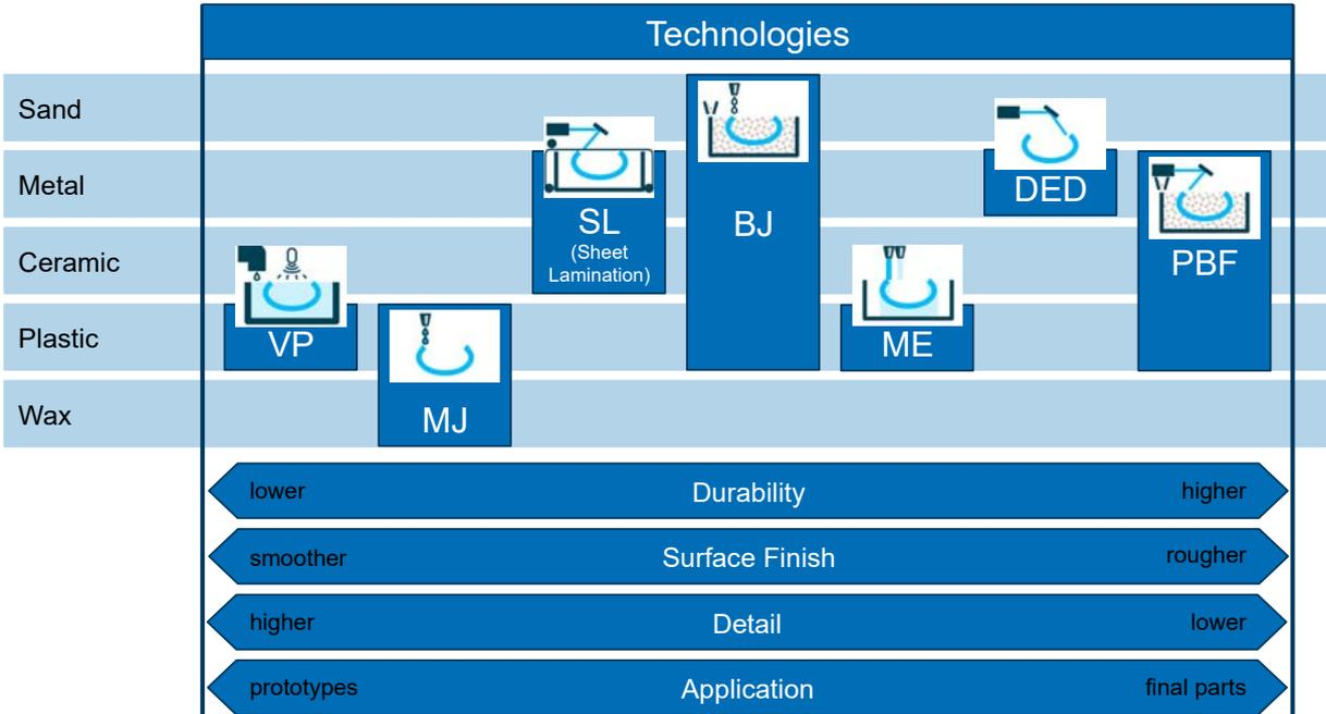
**Figure 2-1: AM technologies and their respective characteristics**
