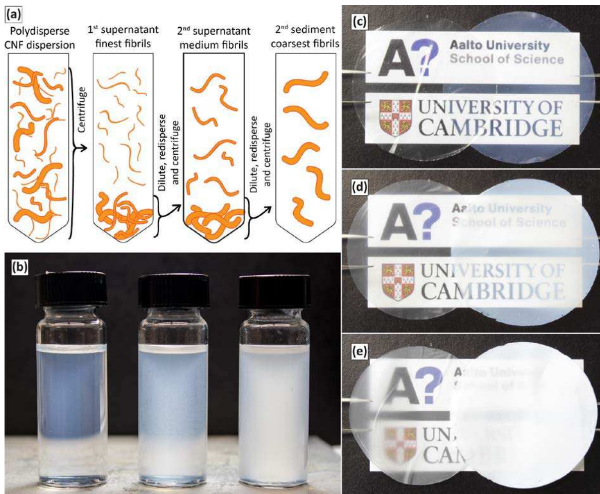
Figure 1. (a) Schematic illustration of the preparation procedure of the fractionated CNF dispersions by differential centrifugation. (b) Photograph of the resulting fractionated CNF dispersions after dilution to an equal concentration (0.9 g / L); left to right: finest, medium and coarsest fibrils. Photographs of the compact CNF films (left) and the \sim 10 \mu\text{m} thick, porous membranes of CNF dried from octane (right) when using (c) the finest, (d) the medium, and (e) the coarsest fibrils. The outer edges of the membranes and the compact films are approximately 1 cm off the paper underneath while the edge at the center of the image is in contact with the paper. In (c) the text remains fully legible underneath the transparent membrane made from the first supernatant, whereas in (e) the text cannot be resolved from under the white membrane fabricated from the coarsest fibrils. The semi-transparent membrane in (d) is the intermediate case. Masses of the compact CNF films and the corresponding porous membranes are 9.43 and 9.35 in (c), 9.53 and 9.11 in (d), and 8.34 and 7.95 mg in (e).
