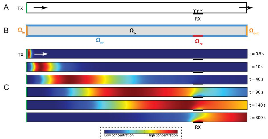
**Fig 1. Microfluidic MC with surface-based receiver.** (A) Conceptual drawing of the system. (B) Domains and boundaries used in the exact system model. (C) Demonstration of concentration-encoded molecular message propagation through the reactive surface of receiver in convection-diffusion channel. Finite element simulations are carried out in COMSOL Multiphysics.
