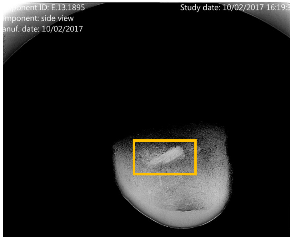
Figure 2-14 - Side view x-ray of E.13.1895 displaying the flat disk of organic material (surrounded by yellow box) resting on the top of the illuminant; x-ray courtesy of Jennifer Marchant
