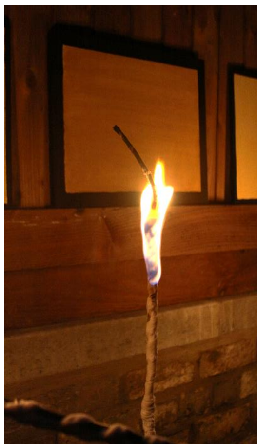
Figure 5-2 - Wick-on-stick device with bent tip after being lit
