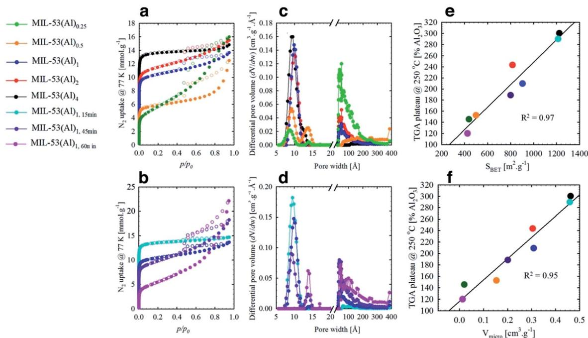
Fig. 4 N<sub>2</sub> isotherms (77 K) and pore size distributions for MIL-53(Al) materials with adjusted modulator stoichiometry/concentration (a and c) and varied reaction time (b and d); linear fits obtained by plotting (e) the BET surface areas ( $S_{\text{BET}}$ ) and (f) micro pore volume ( $V_{\text{micro}}$ ) of all 8 samples against their respective TGA plateau at 250 °C.
