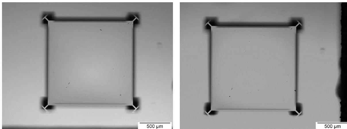
**Figure S-1.** Collection surface (*i.e.* back) of resonator (left) before collecting NaCl particles and (right) before collecting NaCl/MA particles (after using the cleaning method described by Zielinski *et al.*<sup>1</sup>). Images taken with an optical microscope (BX51, Olympus).
