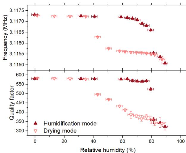
**Figure S-2.** Resonant frequencies (corrected for temperature) and quality factors for AS at each RH across both the deliquescence mode (darker, filled upwards triangles) and the efflorescence mode (lighter, open downwards triangles). Vertical error bars show the range of the five measurements with the quoted value being the average. Horizontal error bars are based on RH uncertainty ( $\pm 2\%$ ).
