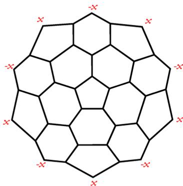
**Figure 11.** Nonzero coefficients (marked  $x$  or  $-x$ ) of the nonbonding MO in *altan*-corannulene (1). All unmarked centers have a zero coefficient in the nonbonding MO. For a normalized MO,  $x = 1/\sqrt{10}$ .
