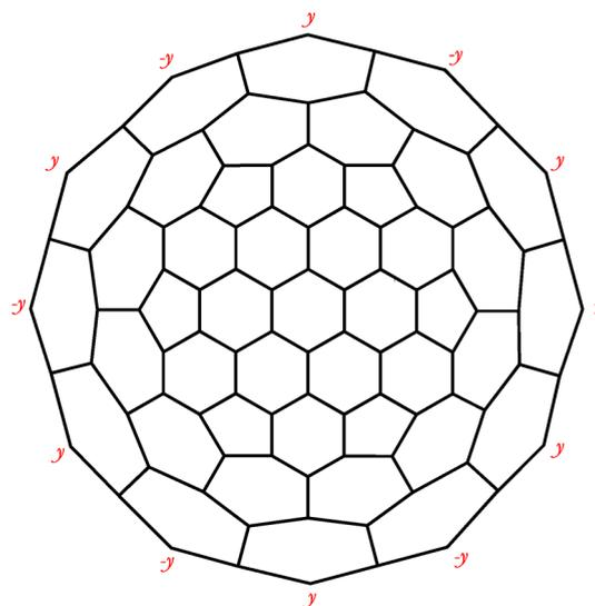
**Figure 12.** Nonzero coefficients (marked  $y$  or  $-y$ ) of the nonbonding MO in (*altan*)<sup>3</sup>-coronene (6). All unmarked centers have a zero coefficient in the nonbonding MO. For a normalized MO,  $y = 1/\sqrt{12}$ .
