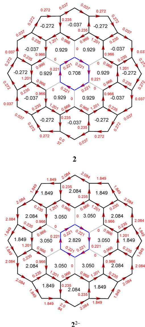
**Figure 5.** Maps for the HLPB topological ring currents (in black) and the associated topological bond currents (in red) for (above) *altan*-coronene (structure **2**, Figure 1; taken from ref 5) and (below) its dianion, **2**<sup>2-</sup>, for comparison. For the conventions on displaying topological ring currents and bond currents, please see the caption to Figure 4.
