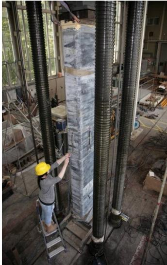
Figure 6 Column strengthening
