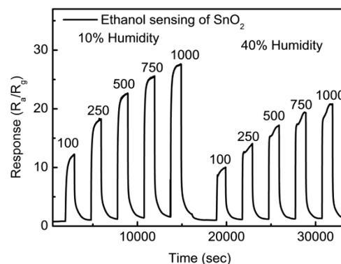
**Fig. 2.** Ethanol sensing at 400 °C of Au-SnO<sub>2</sub> nanocomposites at two different humidity levels. Taken from [8].
