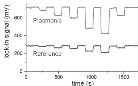
**Fig. 6.** Time-dependent signal obtained from NDIR measurements in a commercial gas sensing setup for the best plasmonic structure ( $2.6 \mu\text{m}$  pitch,  $800 \text{ nm}$  radius) and the thermal emitter without plasmonic crystal structure. Taken from [15].
