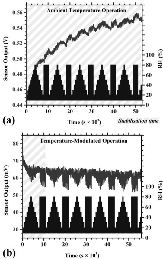
**Fig. 3.** (a) Ambient temperature operation: humidity sensor output as a function of time for different RH levels. (b) Temperature-modulated operation: humidity sensor output as a function of time for different RH levels. Taken from [10].
