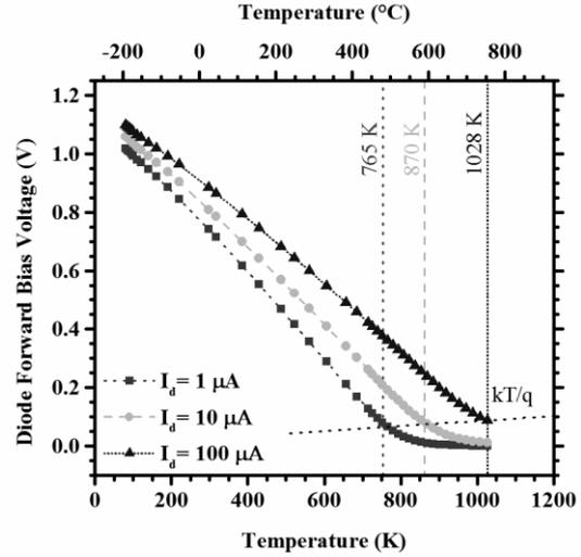
**Fig. 10.** Measured diode forward bias voltage vs. heater temperature of a thermodiode with  $5 \mu\text{m}^2$  junction area for different driving currents (1  $\mu\text{A}$ , 10  $\mu\text{A}$  and 100  $\mu\text{A}$ ). Maximum operating temperatures, obtained equating thermal voltage and diode voltage, are also shown. Taken from [32].
