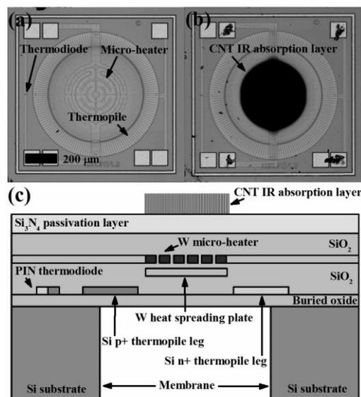
**Fig. 5.** (a) Optical micrograph of the IR detector chip ( $1.6 \text{ mm} \times 1.6 \text{ mm}$ ), (b) optical micrograph of the IR detector chip after CNT radiation absorbing layer in-situ T-CVD growth, (c) schematic cross-sectional depiction of the IR detector. Taken from [13].
