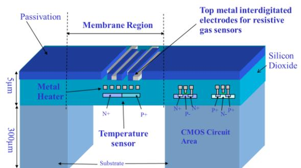
**Fig. 1.** Schematic drawing of an SOI CMOS microhotplate with an integrated thermodiode and CMOS cells outside the membrane. In this schematic drawing the micro-hotplate features top electrodes and a sensitive layer for gas-sensing or humidity detection.
