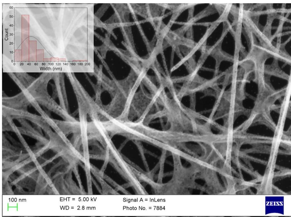
*Figure S-1: SEM of calcined nanofibres.*
