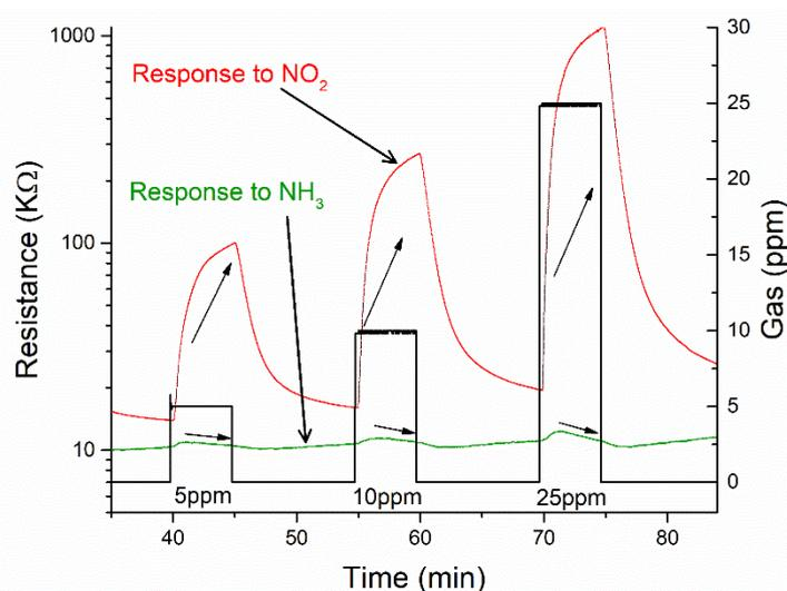
Figure S-6: Red (Green) curve is the response of the ZnO sensor to the  $\text{NO}_2$  ( $\text{NH}_3$ ) gas. Black curve shows the concentration of the gases-  $\text{NH}_3$  and  $\text{NO}_2$ . These two experiments are done seperately but drawn together for comparison.
