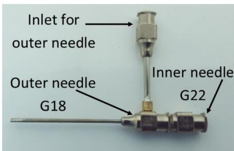
*Figure S-2: Photograph of a coaxial needle used in this experiment.*
