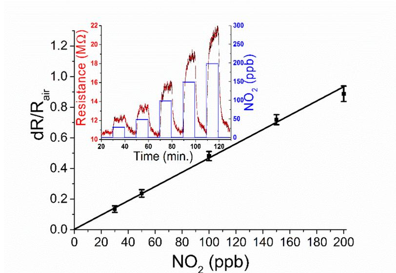
Figure S-4: Sensitivity of the ZnO nanofibre device containing fewer fibres than the results presented in Figure 3f.
