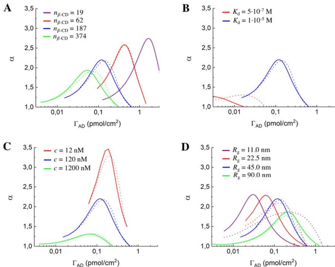
**Fig. S6. Analytical modeling at tunable polymer characteristics.** Superselectivity parameter,  $\alpha$ , extracted from the theoretical data show in Fig. 6B-E and plotted vs  $\Gamma_{\text{AD}}$ . Analytical predictions are obtained for the fluid (solid) and immobile (dashed) cases at tunable  $n_{\beta\text{-CD}}$  (A),  $K_d$  (B),  $c$  (C) and  $R_g$  (D). Blue curves in all graphs correspond to the reference system (Table 1).
