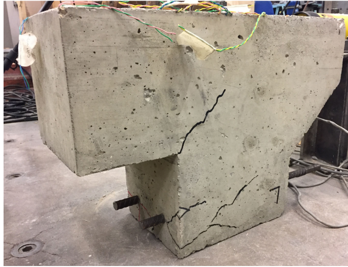
Figure 5. Cracking pattern for test A16-C50-50-a.
