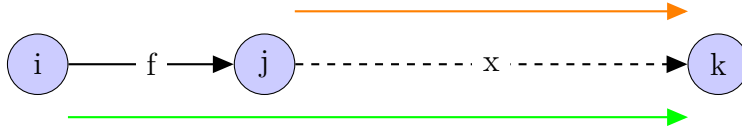
Figure 4.2: The (strictly) increasing condition says that f(x) , the result of extending x , must always be worse than x itself.
