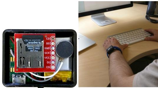
Figure 3.4: Electronics (left) enclosed in 3D printed box (3x4x1.5cm) and complete prototype attached to velcro wristband (right).
