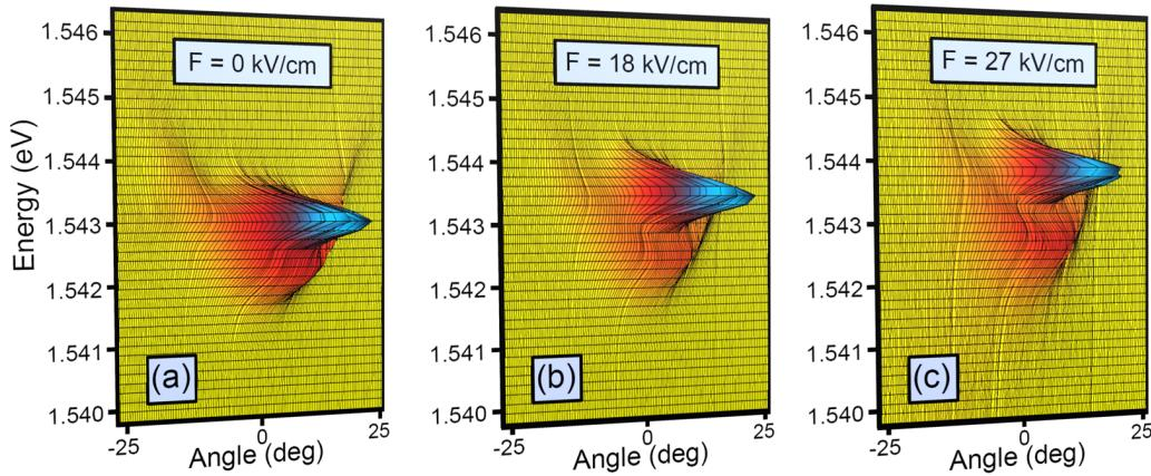
FIG. 2. Angle-dependent polariton far-field emission under nonresonant continuous wave excitation recorded on the logarithmic scale. A gradual blueshift of polariton condensate energy is observed when the electric field is applied: (a) zero bias, (b) 18 kV/cm, and (c) 27 kV/cm. Superimposed weak emission arising from noncondensed low-excitation density areas of the sample surrounding the central spot shows a similar energy blueshift.
