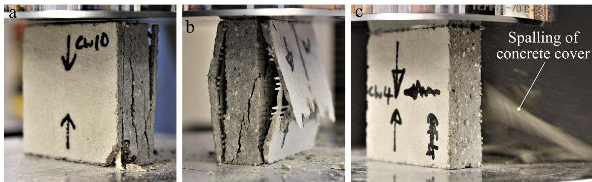
Figure 5.20: TRC samples tested in compression, showing a) typical crack pattern after failure (Shell 3), b) splitting in the reinforcement plane (Shell 1) and c) spalling of the cover layer before failure (Shell 2).
