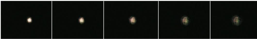
Figure 118 Captured images of 50  $\mu\text{m}$  MMF output beam profiles along the propagation distance.
