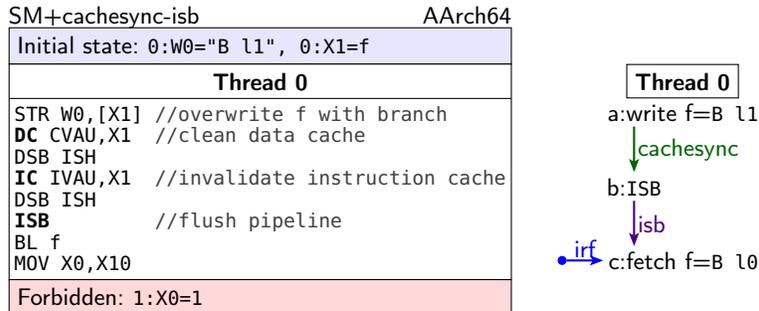
Now the outcome is forbidden. The cache synchronisation sequence `DC CVAU; DSB ISH; IC IVAU; DSB ISH` (which we abbreviate to a single `cachesync` edge) ensures that by the time the `ISB` executes, the instruction and data memory have been made coherent with each other for `f`. The `ISB` then ensures the final fetch of `f` is ordered after this sequence. The microarchitectural intuition for this was in §2; our §4 operational model will describe the semantics of each instruction.
