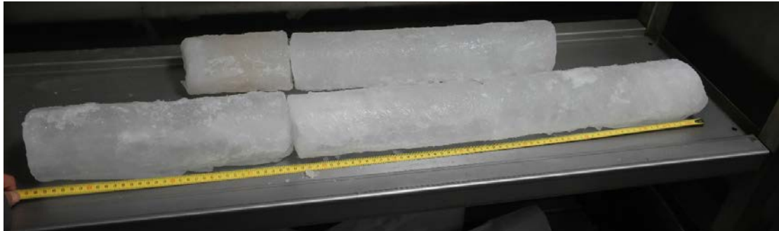
(a) Case A - Ice core 3 in the -20^{\circ}\text{C} freezer laboratory: Thin sectioning, 156 cm ice, 60 cm snow, centre sample location.
