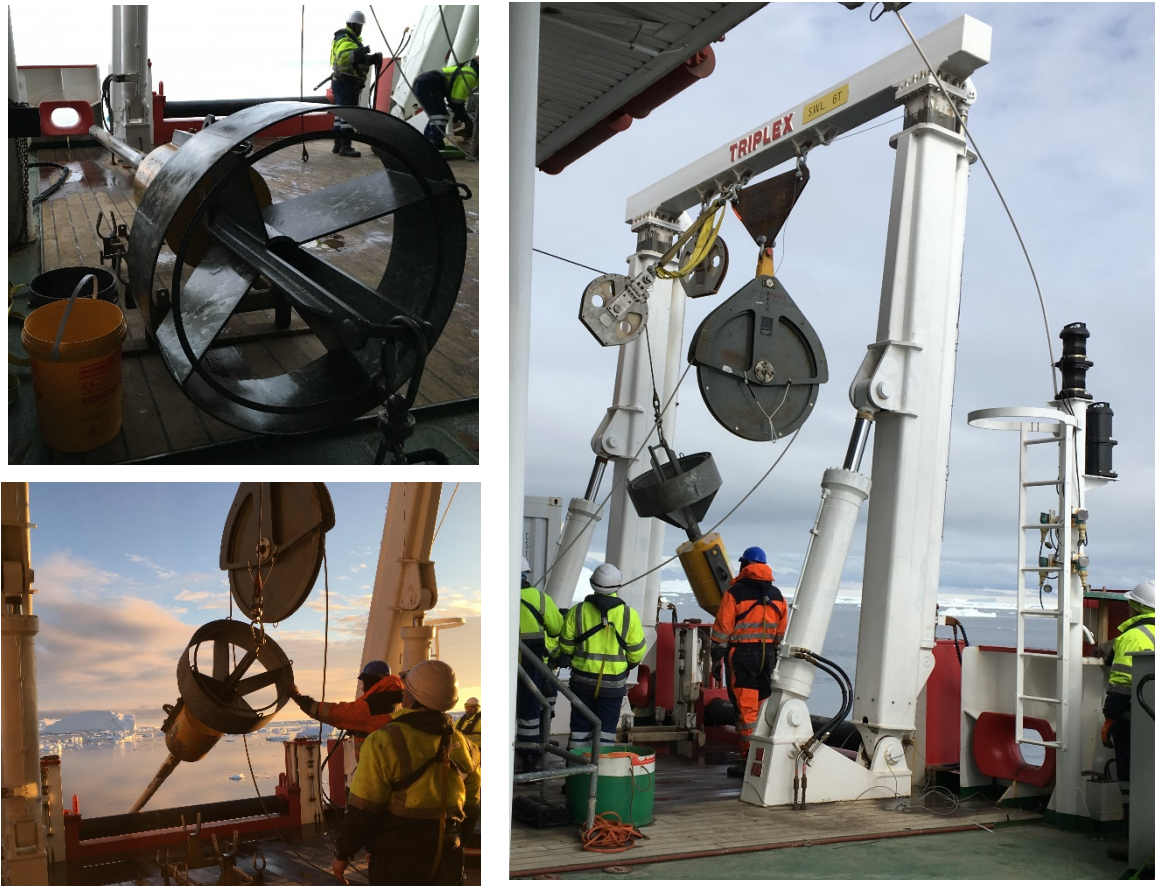
Figure 5.2. The gravity core is seen here with a 6 m core barrel being winched over the back of the SA Agulhas II .
