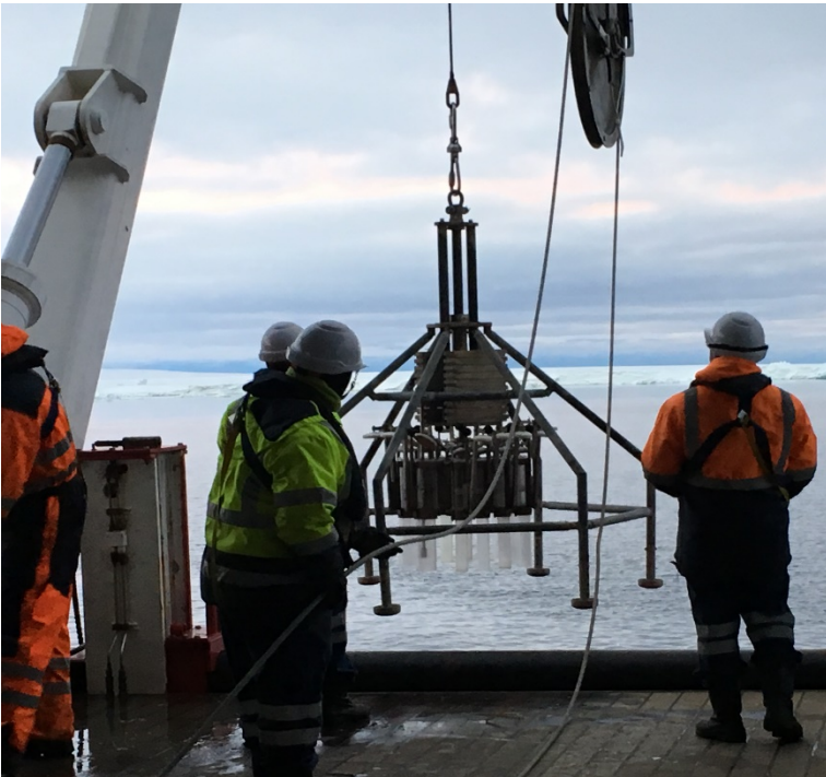
Figure 5.3. The multi-corer being deployed by winch over the stern of the SA Agulhas II.
