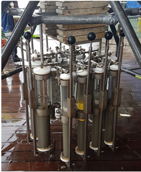
Figure 7.11. (a) Multi Corer back on deck (b) Dense phytoplankton floc on the surface of a core
