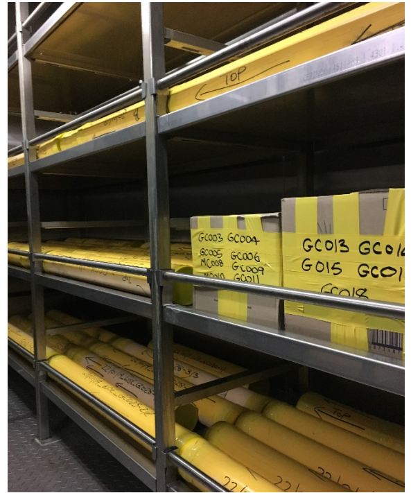
Figure 5.4. Cores were cut into 1 m lengths, labelled and placed in cold storage on board. Splitting and analysis will take place at BOSCORF, UK.
