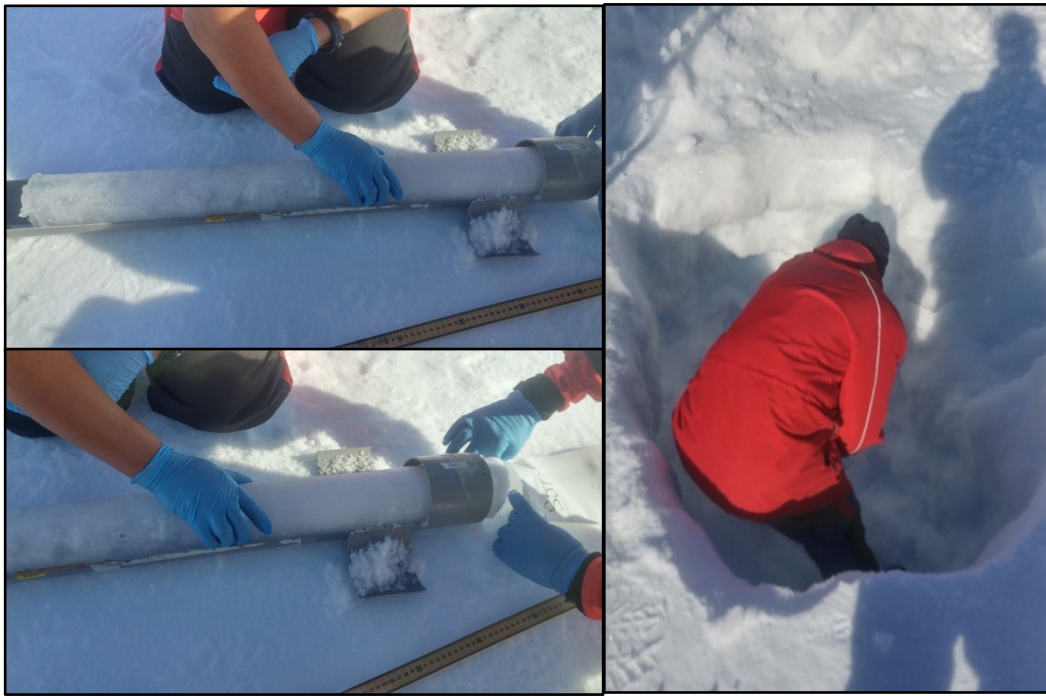
Figure 7.14. Anticlockwise from right: Snow pit being dug by one of the scientists involved in sampling; ice core resting in a PVC cradle where both length and temperature were measured; sea ice core being bagged for transport and storage.
