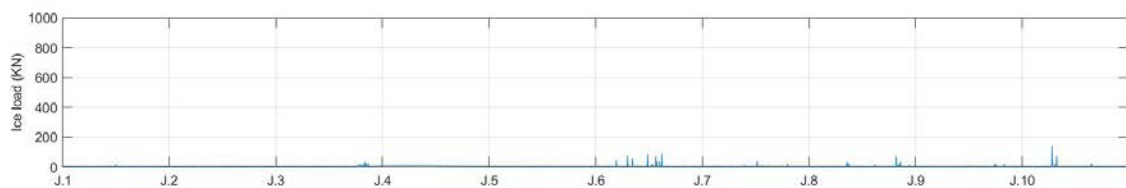
Figure 9.5. Ice loads measured on three structural frames on the starboard side of the bow shoulder for 1 to 10 January.
