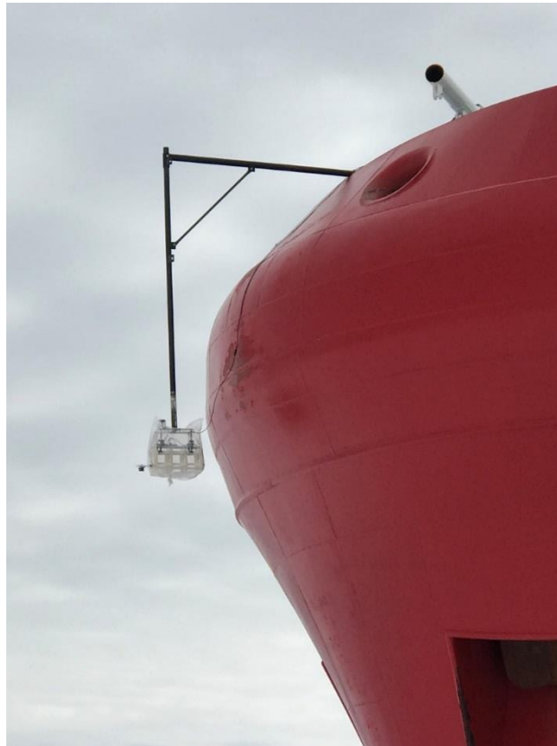
Figure 6.15. Drone snow radar mounted on the ship's bow of SA Agulhas II for a pilot study to measure snow thickness over sea ice.
