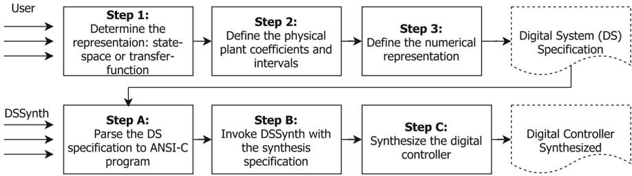
**Fig. 5** The digital-system synthesizer (DSSynth) tool—distinct phases of the controller synthesis
