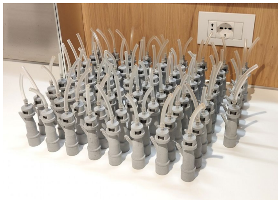
Figure 1. 3D printed ventilator valves © Isinnova.
