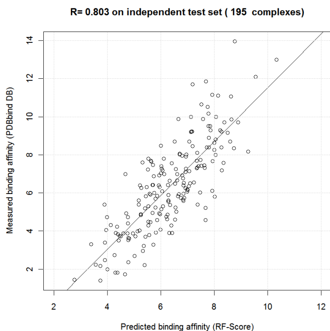
Figure 8: RF-Score::Elem-v2 predicted versus measured binding affinity on the independent test set (195 complexes). Pearson's correlation coefficient R_p=0.803 , Spearman's correlation coefficient R_s=0.797 , standard deviation SD = 1.54 \log K_{d/i} units and Root Mean Square Error RMSE = 1.53 \log K_{d/i} units. This plot can be visually compared to those for the best performing scoring functions in Cheng et al. 41 's figure 6. Performance comparisons on the same test set are presented here in figure 9.
