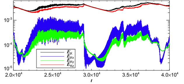
**Figure 9.** Kinetic energies as a function of time in a regime that fluctuates between wave turbulence and zonal flows. Simulation parameters are  $R = 0.01$ ,  $Pe=4\pi^2$ ,  $Re=10^{5.5}$ .
