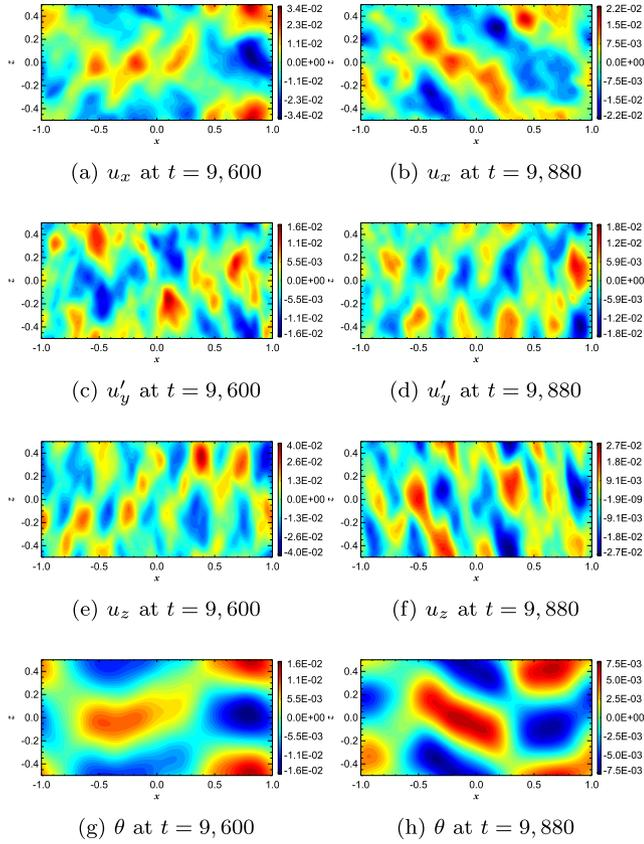
**Figure 7.** Plots of  $u_x$ ,  $u'_y$ ,  $u_z$ , and  $\theta$  in  $x$ - $z$  space at two times for a run showing wave turbulence. Simulation parameters are  $R = 0.01$ ,  $Pe=4\pi^2$ ,  $Re=10^{5.25}$ .
