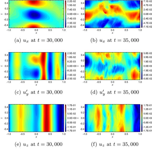
**Figure 10.** Plots of  $u_x$ ,  $u'_y$ , and  $u_z$  in  $x$ - $z$  space at two times for a run exhibiting intermittent zonal flows (left-hand panels) that emerge from periods of pure wave turbulence (right-hand panels). Simulation parameters are  $R = 0.01$ ,  $Pe=4\pi^2$ ,  $Re=10^{5.5}$ .
