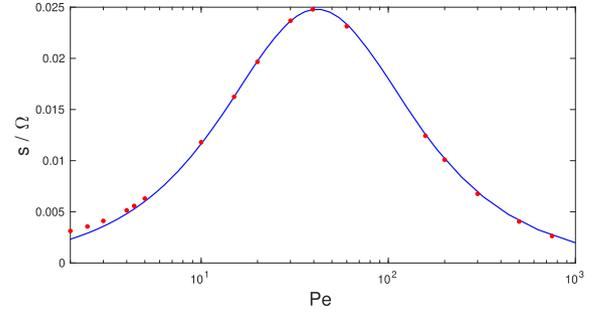
**Figure 1.** Linear growth rate of the COS mode  $s$  as a function of  $Pe$ , for  $R = 0.1$  and  $Re = 2 \times 10^5$ . The solid blue curve represents the analytic solution; the red dots are numerically calculated values.
