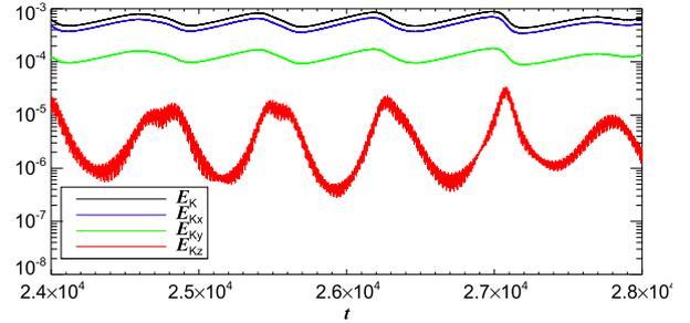
**Figure 3.** Kinetic energy, and its separate components, as a function of time bandpass filtered to remove highest frequency oscillations. Simulation parameters are  $R = 10^{-1.5}$ ,  $Pe=4\pi^2$ ,  $Re=10^{3.75}$ .
