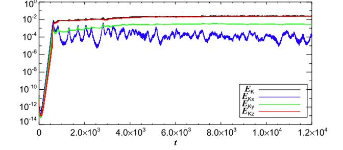
**Figure 11.** Kinetic energies as a function of time in a regime containing strong, persistent zonal flows. Simulation parameters are  $R = 0.1$ ,  $Pe=4\pi^2$ ,  $Re=10^{5.5}$ .
