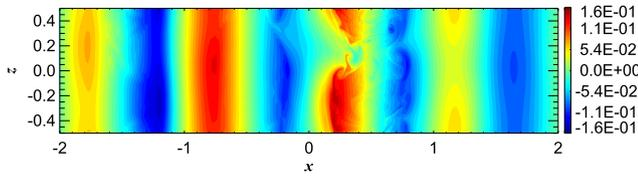
**Figure 14.** Plot of  $u'_y$  in  $x$ - $z$  space for a run with  $L_x = 4L_z$  that displays persistent zonal flows in its saturated state. Simulation parameters are  $R = 0.1$ ,  $Pe=4\pi^2$ ,  $Re=2 \times 10^5$ .
