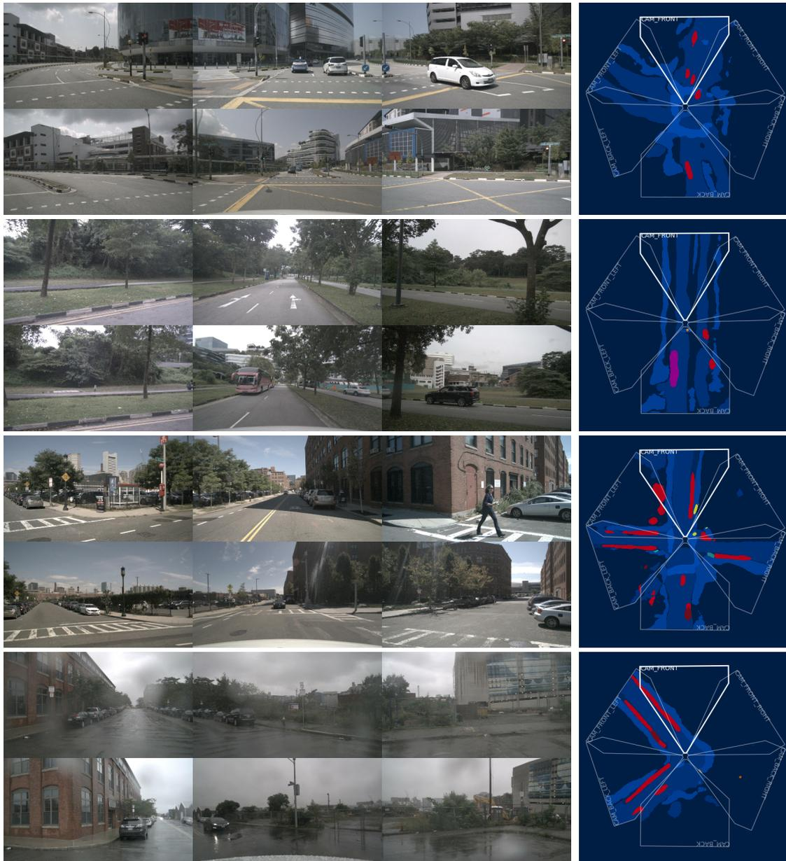
Figure 4.11. Composite local maps (right) generated by applying Bayesian filtering to images from six surround-view cameras (left).
