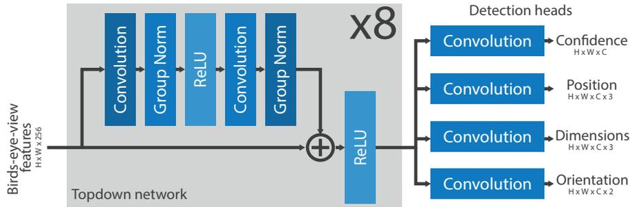
Figure 3.5. Illustration of the topdown network architecture and detection heads. The topdown network consisted of a sequence of 8 residual units derived from the basic blocks of He, Zhang, et al. (2016).
