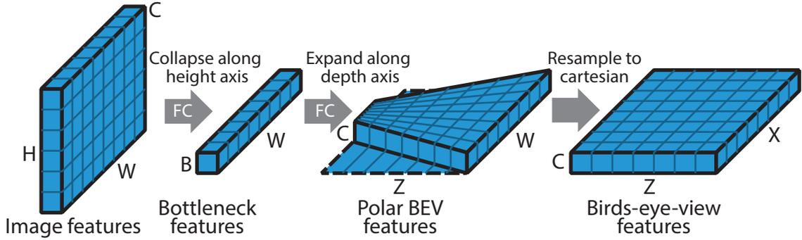
Figure 4.3. The Dense Transformer Layer. (1) Each column of the image was encoded to a single feature vector. (2) The column features were expanded along camera rays in the birds-eye view. (3) The non-Cartesian feature map was resampled into a Cartesian coordinate system, to give a single feature per birds-eye view location.
