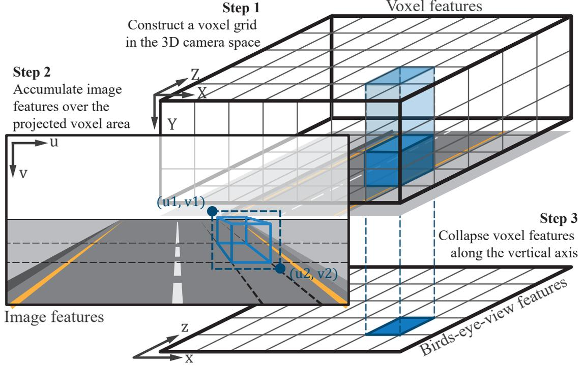
Figure 3.3. Overview of the Orthographic Feature Transform (OFT). The transform consists of three steps: (1) A voxel grid is constructed which spans the 3D space of interest. (2) The voxel feature  $\mathbf{f}_{ijk}^{vox}$  is computed by projecting the voxel into the image, and accumulating image features over the region defined by bounding box  $(u_1, v_1, u_2, v_2)$ . (3) birds-eye view feature  $\mathbf{f}_{pq}^{bev}$  is computed by accumulating voxel features along the vertical axis.
