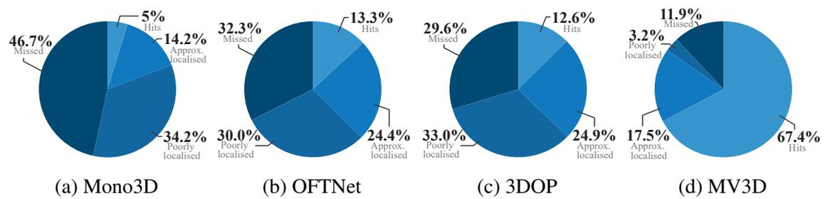
Figure 3.12. Breakdown of detection and localisation errors in object detection algorithms. Clockwise from the top, the shaded regions represent the proportion of detections which were correctly detected (‘hits’), detected but not accurately localised, detected but poorly localised, and not detected.
