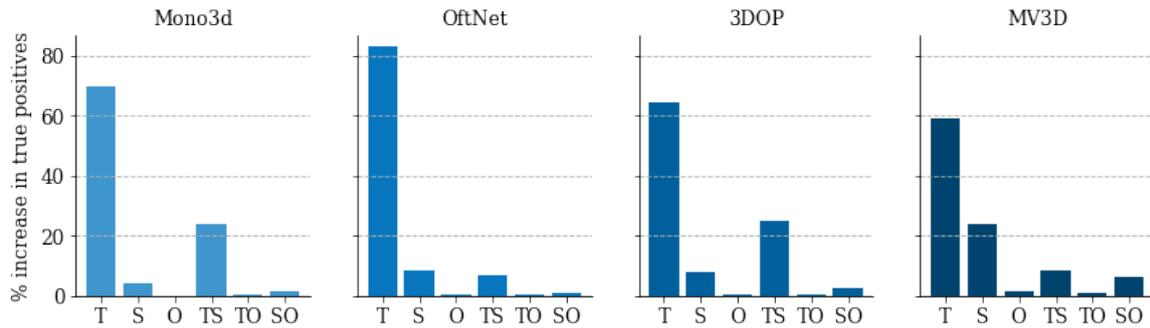
Figure 3.17. Percentage improvement in true-positive detections when translation, scale or orientation predictions are corrected to their ground truth value. T - translation, S - scale, O - orientation, TS - translation and scale, TO - translation and orientation, SO - scale and orientation.
