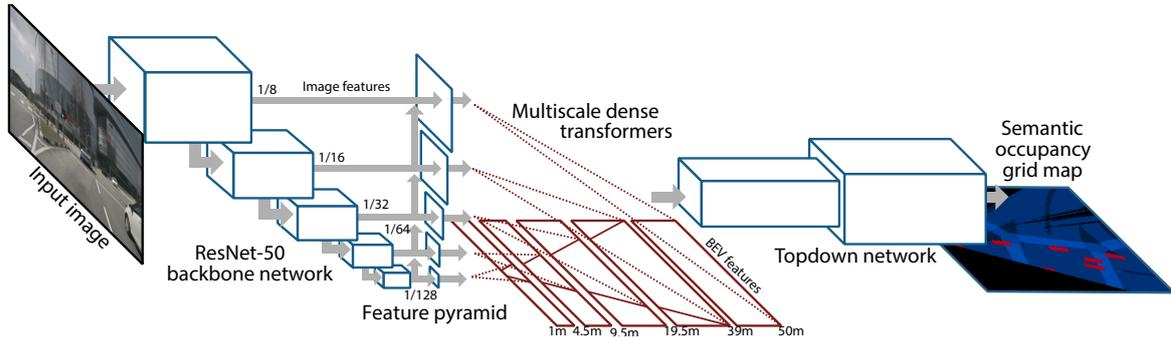
Figure 4.1. Overview of the Pyramid Occupancy Network architecture.
