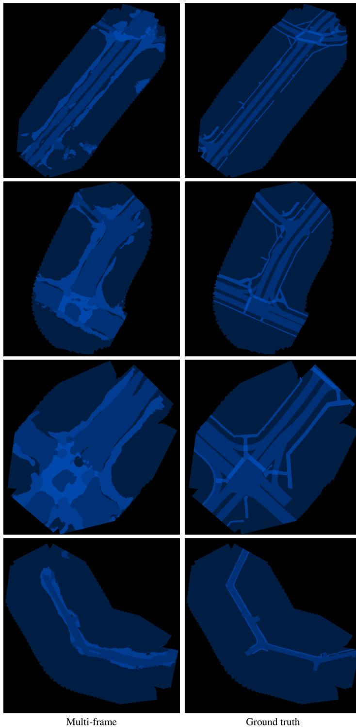
Figure 4.9. Examples of large-scale maps from the NuScenes validation set. The left column shows maps generated by applying the Bayesian filtering algorithm described in Section 4.2, using a calibrated PyrOccNet network as the inverse sensor model. The right column shows the corresponding ground truth map. Only the four static NuScenes classes (*drivable area*, *walkway*, *pedestrian crossing* and *parking space*) are shown. See Figure 4.10 for a comparison to single-frame results.
