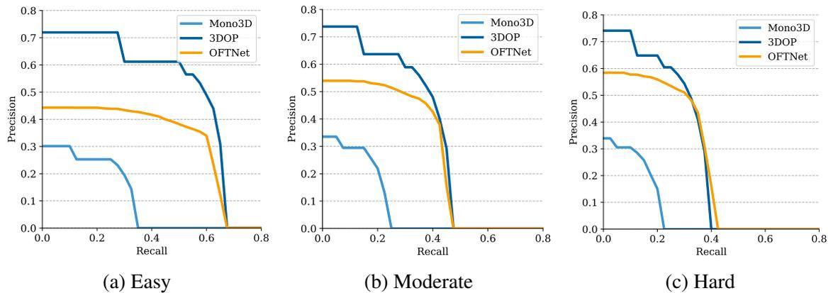
Figure 3.10. Precision-recall curves on the KITTI validation set for the Mono3D (Chen, Kundu, Zhang, et al., 2016), 3DOP (Chen, Kundu, Zhu, et al., 2015) and OFTNet algorithms. To better differentiate between the three methods, we use a more lenient IoU threshold of 50% to determine true positive predictions.
