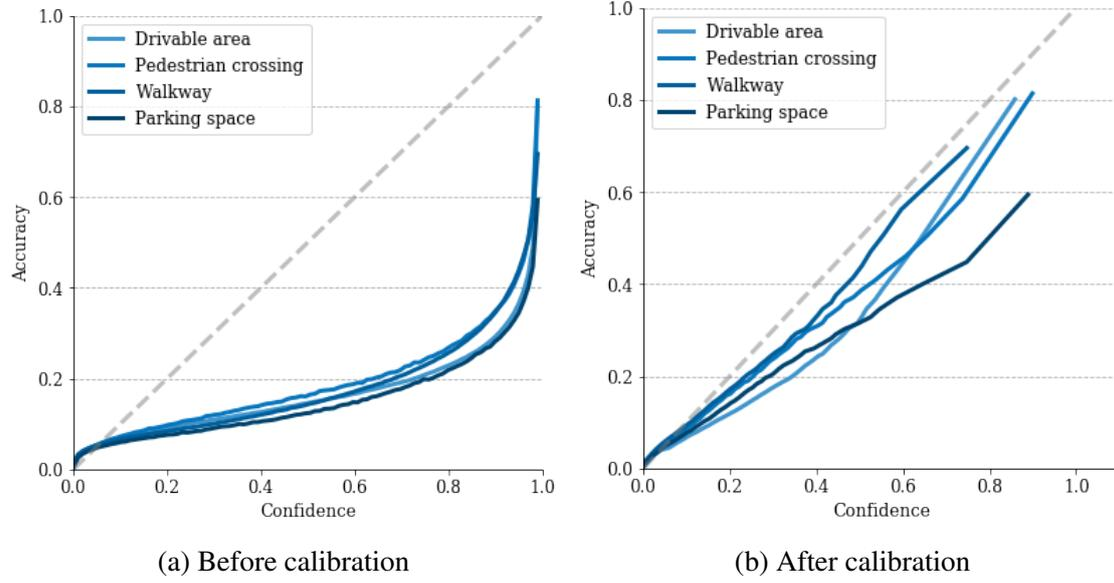
Figure 4.8. Reliability diagrams showing model accuracy against confidence, evaluated on the NuScenes validation set. Dashed line represents a perfectly calibrated model.
