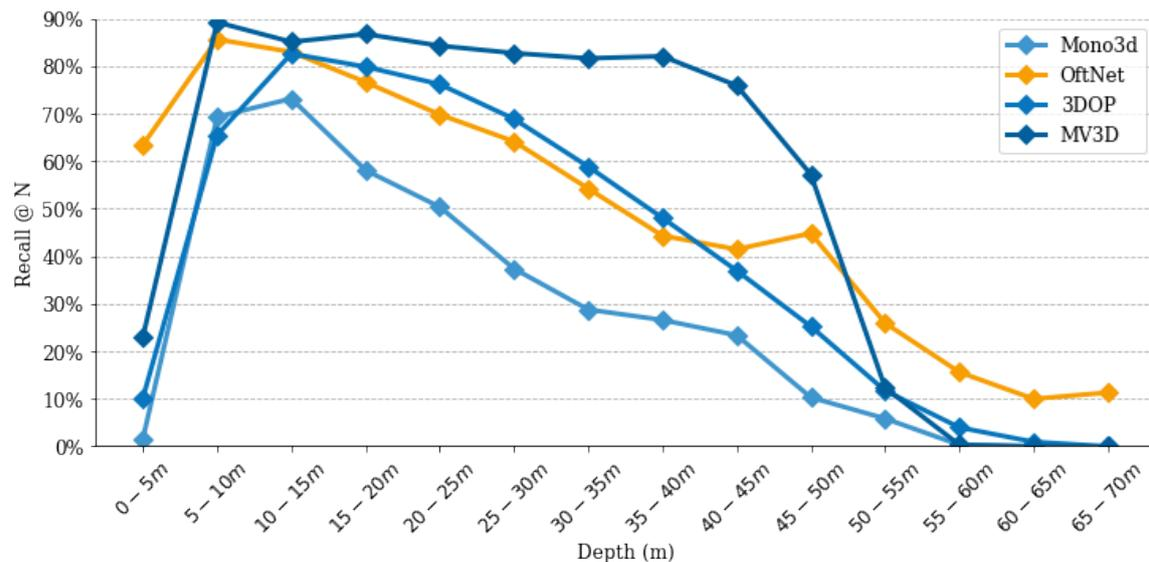
Figure 3.13. Top  $N$  recall as a function of distance of the object centre away from the camera.
