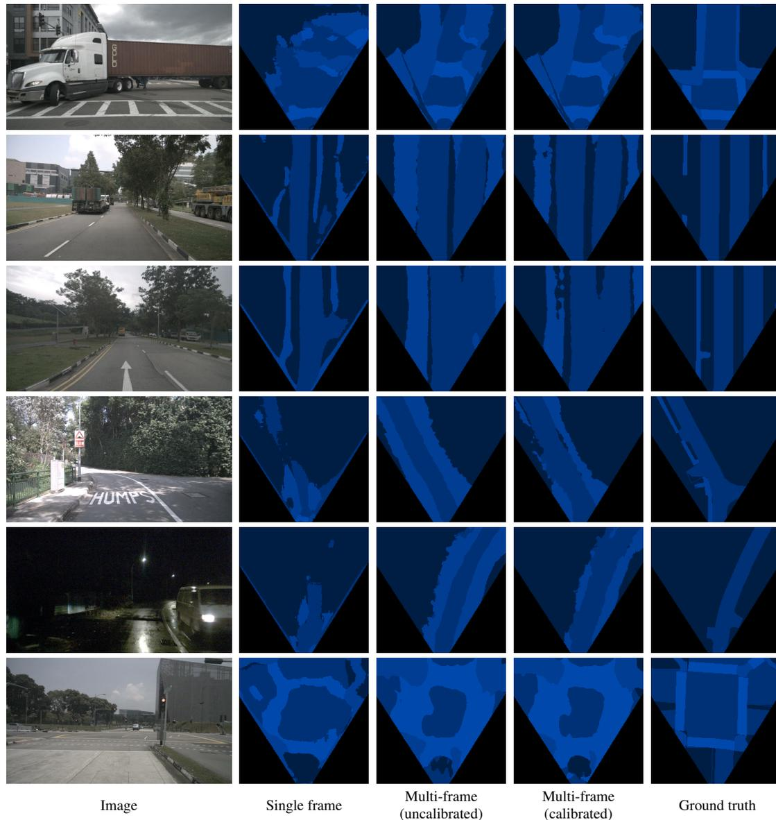
Figure 4.10. Qualitative comparison of single-frame vs multi-frame fusion methods on the NuScenes validation set. Multi-frame results are warped back into the single-frame field of view for comparison.
