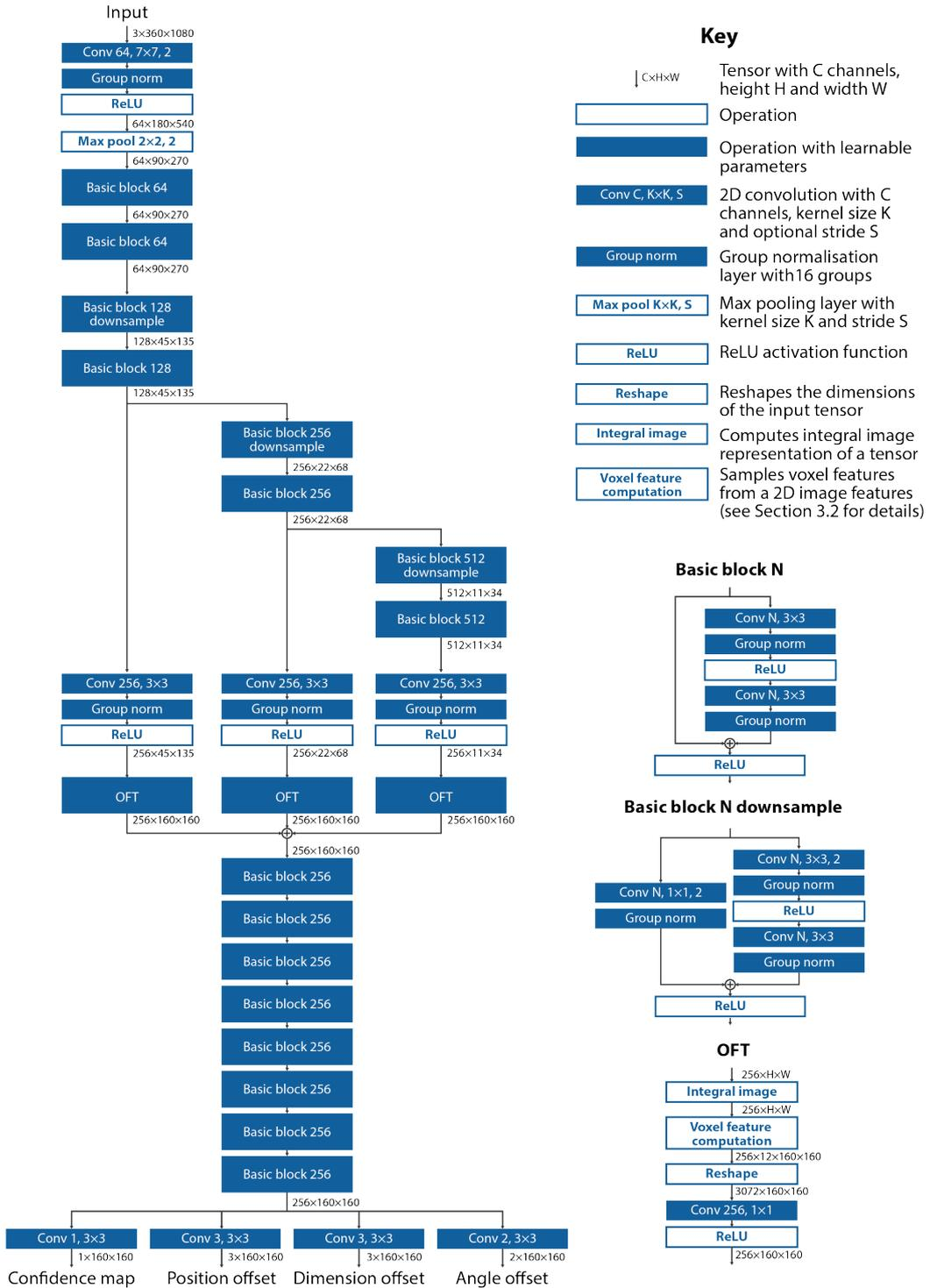
Figure 3.7. A complete specification of the OFTNet architecture. Filled blocks represent neural network layers with trainable parameters. Descriptions of submodules within the network, consisting of the residual basic block (He, Zhang, et al., 2016), residual basic block with downsampling, and orthographic feature transform, are shown on the right.
