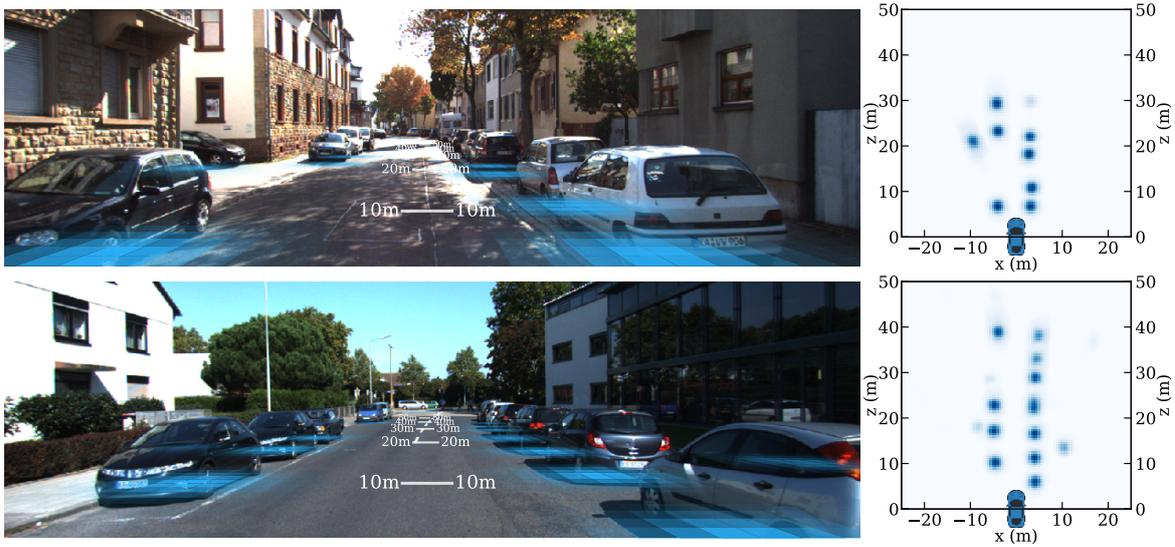
Figure 3.6. Examples of confidence maps for the car class predicted by our approach. The image on the right shows the predicted peaks in the birds-eye view, while the image on the left shows their corresponding projection onto the ground plane. Note that the ground plane is used only for visualisation and is not an input to our approach.
