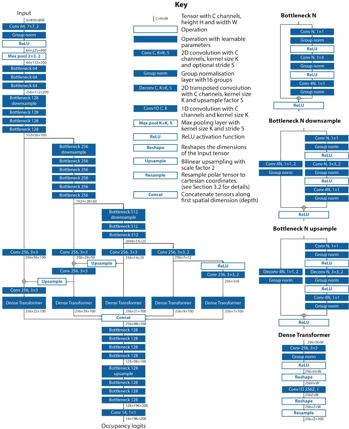
Figure 4.4. A complete specification of the Pyramid Occupancy Network architecture. Filled blocks represent neural network layers with trainable parameters.
