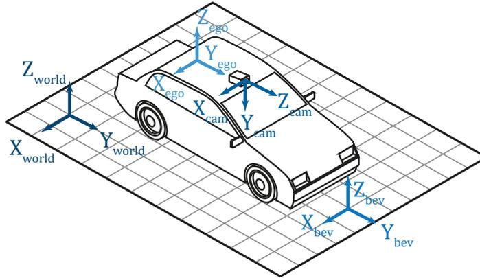
Figure 3.2. Overview of the four main coordinate systems considered in this thesis.
