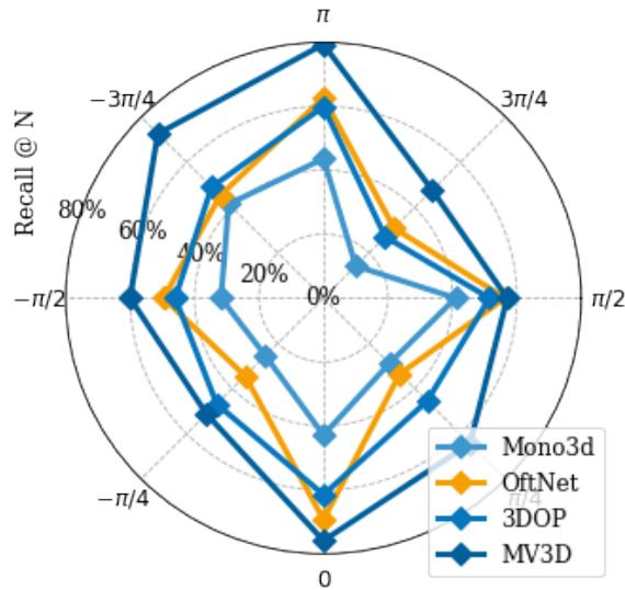
Figure 3.14. Top  $N$  recall as a function of orientation. Zero radians represents objects facing directly towards the camera, while  $\pm\pi$  radians represents objects facing directly away.
