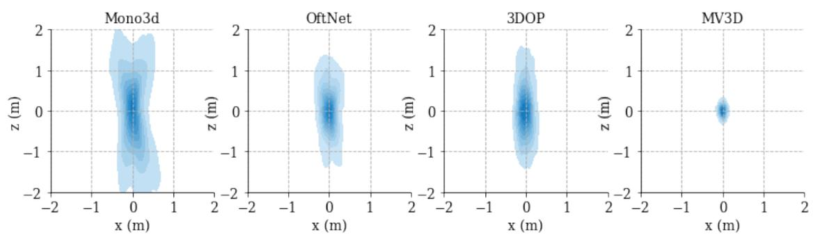
Figure 3.19. Kernel density estimate showing the distribution of position errors in the birds-eye view XZ-plane.
