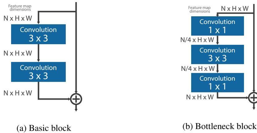
Figure 4.2. Comparison between the two types of residual block used in the ResNet-18 and ResNet-50 feature extractors.  $K \times K$  indicates the size of the convolutional kernel.  $N$  is the number of feature channels, and  $H \times W$  indicates the spatial dimensions of the feature map.
