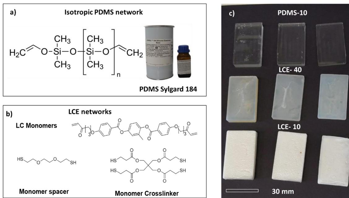
Fig. S1. Preparation of damping materials. (a) Isotropic PDMS network (b) LCE networks (c) pictures of the resulting materials.
