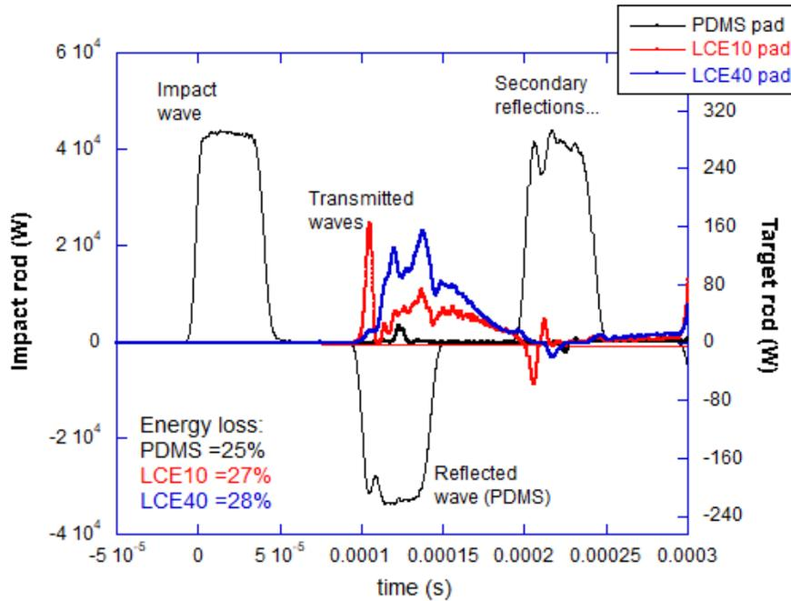
Fig. S4. The split Hopkinson bar impact on a flat-face cylinder elastomer pad. The impact energy is 2J, with 25-28% of impact energy absorbed in the elastomers.
