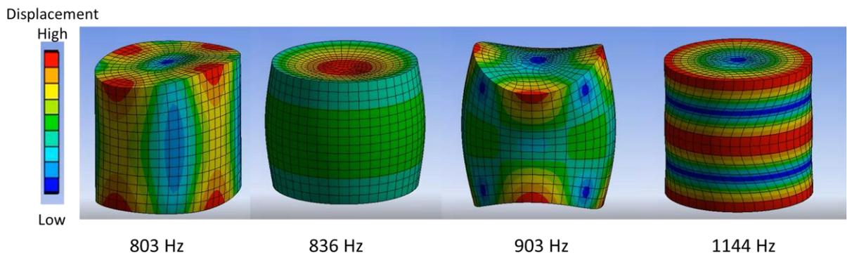
Fig. S7. Mode shape analyses of a typical liquid crystal cylinder.
