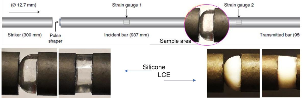
Fig. S3. Schematic of the design. The striker bar generates a compression wave in the incident bar, the shape of which is recorded by the strain gauge 1, first in passing towards the impact, and then in reflection. After the impact, the transmitted mechanical energy forms the compression wave travelling along the target (transmitted) bar, which is recorded by the strain gauge 2.
