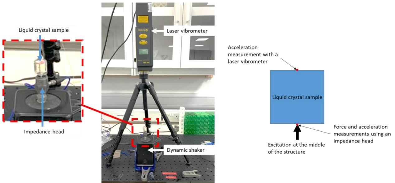
Fig. S6. Illustration of the vibrometer setup, with the acoustic transducer at the bottom of the cylindrical sample, and the laser range meter at the top.
