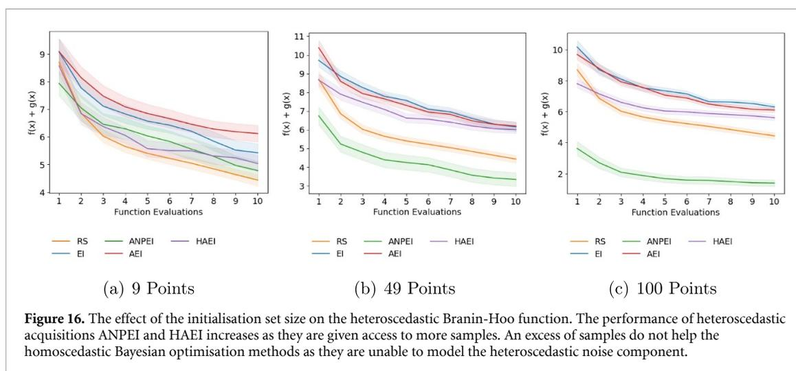
**Figure 16.** The effect of the initialisation set size on the heteroscedastic Branin-Hoo function. The performance of heteroscedastic acquisitions ANPEI and HAEI increases as they are given access to more samples. An excess of samples do not help the homoscedastic Bayesian optimisation methods as they are unable to model the heteroscedastic noise component.
