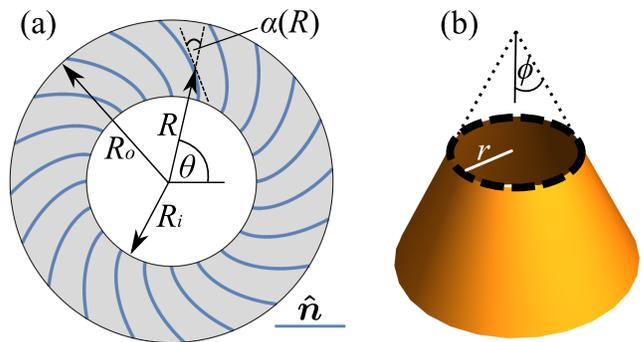
Figure 1. (a) An annular LCE sheet in the reference domain, with an axisymmetric spiral director pattern characterized by the angle  $\alpha(R)$ . (b) A truncated cone with semi-angle  $\phi$ . The dashed circle has curvature  $1/r$ , and geodesic curvature  $k_g$  of magnitude  $\sin(\phi)/r$ .
