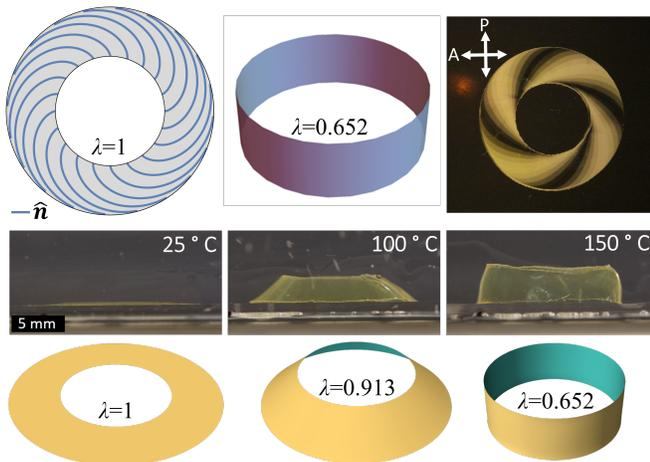
Figure 3. Director spiral (top-right) to morph an annulus into a cylinder (top-middle) at a design  $\lambda = 0.652$ . Experiments (middle) and numerics (bottom) confirm the cylinder is attained, and also highlight the intermediate cone states en route.
