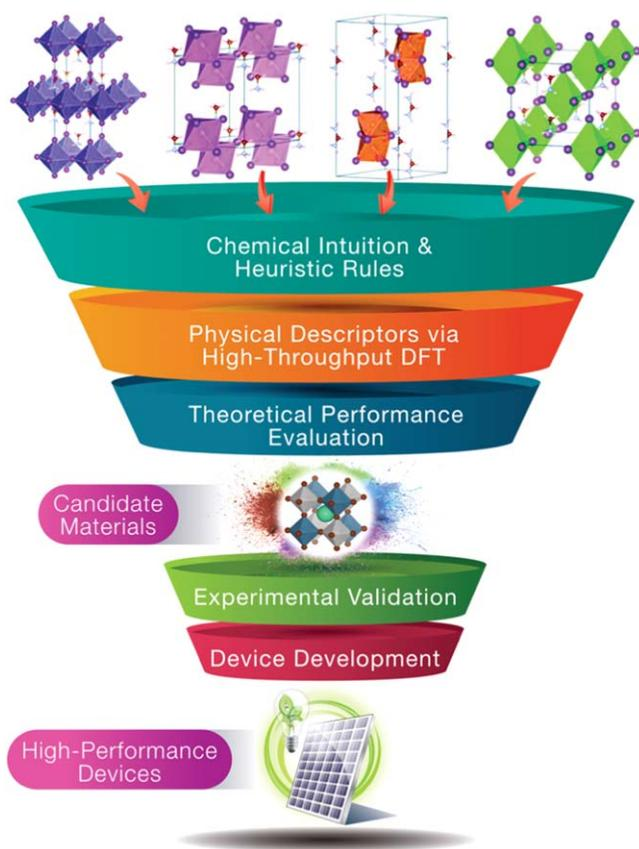
**Figure 2.** Simplified procedural outline of a typical high-throughput screening investigation, with a large input material space reduced to a small selection of promising candidates for further experimental verification and device development.
