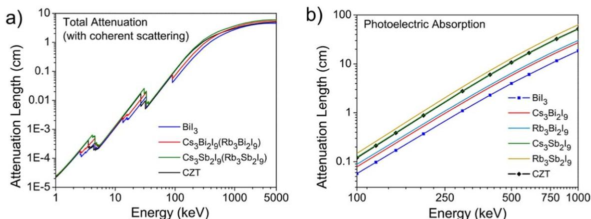
**Figure 25.** Attenuation length of perovskite-inspired materials compared to  $\text{Cd}_x\text{Zn}_{1-x}\text{Te}$  (CZT) under (a) total attenuation and (b) photoelectric absorption. Reprinted with permission from [429]. Copyright (2018) American Chemical Society.
