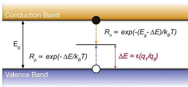
**Figure 5.** Electronic energy diagram of Shockley–Read–Hall recombination at a defect level  $\Delta E = \varepsilon(q_1/q_2)$  above the valence-band maximum (VBM) (More on charge transition levels in section 2.3.3). Electron and hole capture rates,  $R_n$  and  $R_p$ , are exponentially dependent on the energy separation between trap level and band-edge.
