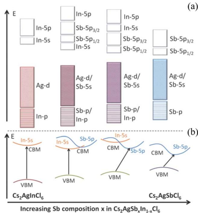
**Figure 16.** (a) Model band diagrams for  $\text{Cs}_2\text{AgSb}_x\text{In}_{1-x}\text{Cl}_6$  and (b) illustration of how the band gap changes due to the contributions from In 5s and Sb 5p orbitals in the conduction band. Reproduced from [241] with permission of The Royal Society of Chemistry.
