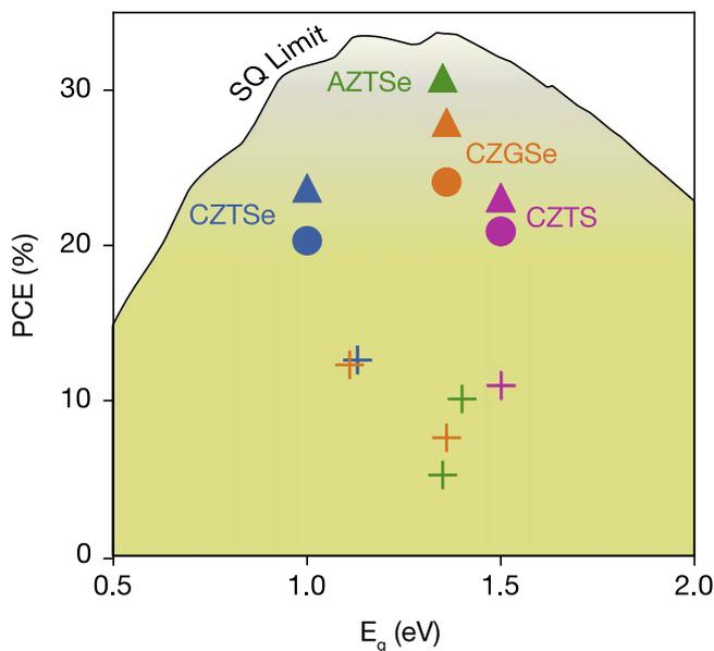
**Figure 4.** Shockley–Queisser limit and trap-limited-conversion (TLC) efficiencies for the kesterite family of thin-film PV materials. Filled symbols represent the TLC power-conversion efficiency and the black line is the SQ limit. TLCs with doping (triangles) show improved performances over TLCs without doping (circles). Plus signs indicate experimental data for kesterite solar cells. Reproduced from [44]. CC BY 3.0.
