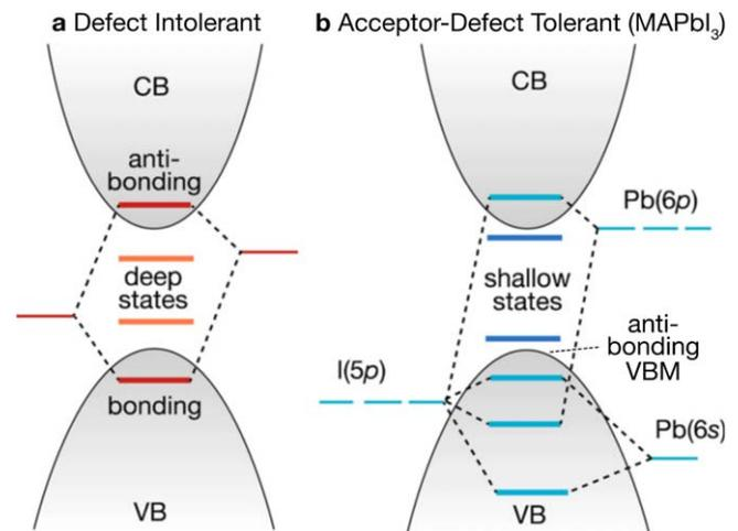
**Figure 6.** Electronic structure of typical ‘defect intolerant’ III–V, II–VI, or group IV semiconductors (left), prone to the formation of deep defect levels, compared to the ‘defect tolerant’ anti-bonding valence band of the lead halide perovskites (right). Reprinted with permission from [18]. Copyright (2017) American Chemical Society.
