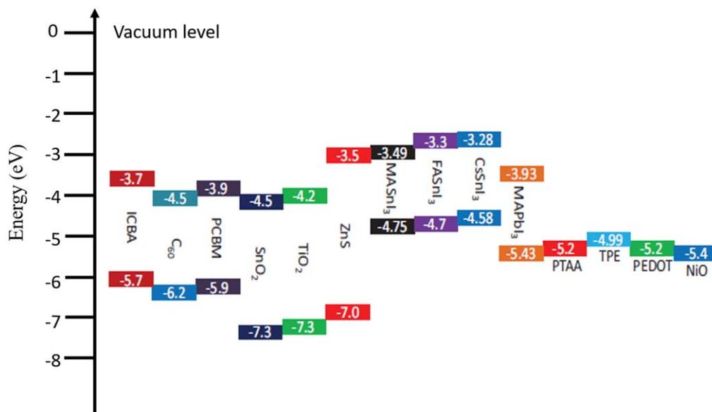
**Figure 20.** Energy diagram of Sn- and Pb-based perovskites along with some common ETLs and HTLs. Unit is in eV. The energy levels are estimated from Tauc plots and photoemission spectroscopy in air. [19] John Wiley & Sons. © 2018 WILEY-VCH Verlag GmbH & Co. KGaA, Weinheim.
