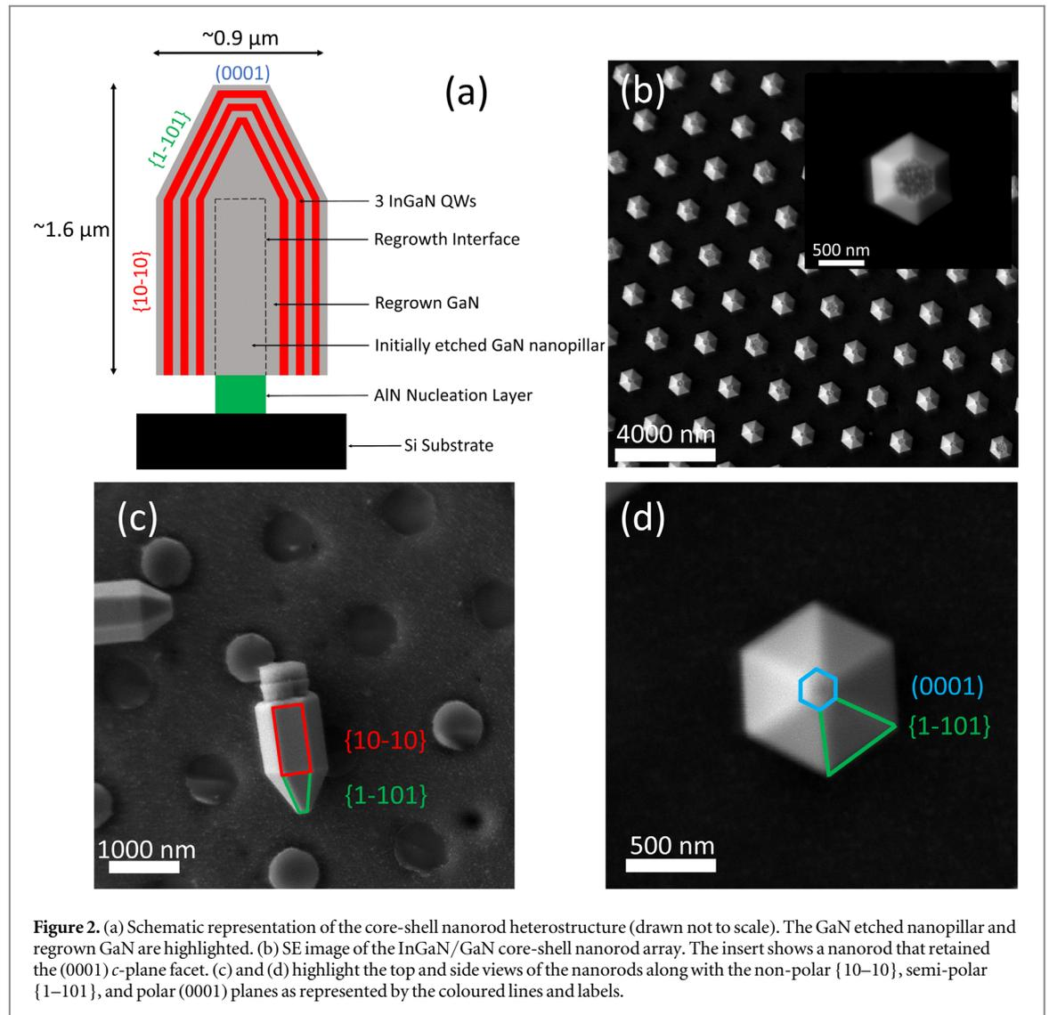
**Figure 2.** (a) Schematic representation of the core-shell nanorod heterostructure (drawn not to scale). The GaN etched nanopillar and regrown GaN are highlighted. (b) SE image of the InGaN/GaN core-shell nanorod array. The insert shows a nanorod that retained the (0001) *c*-plane facet. (c) and (d) highlight the top and side views of the nanorods along with the non-polar {10–10}, semi-polar {1–101}, and polar (0001) planes as represented by the coloured lines and labels.
