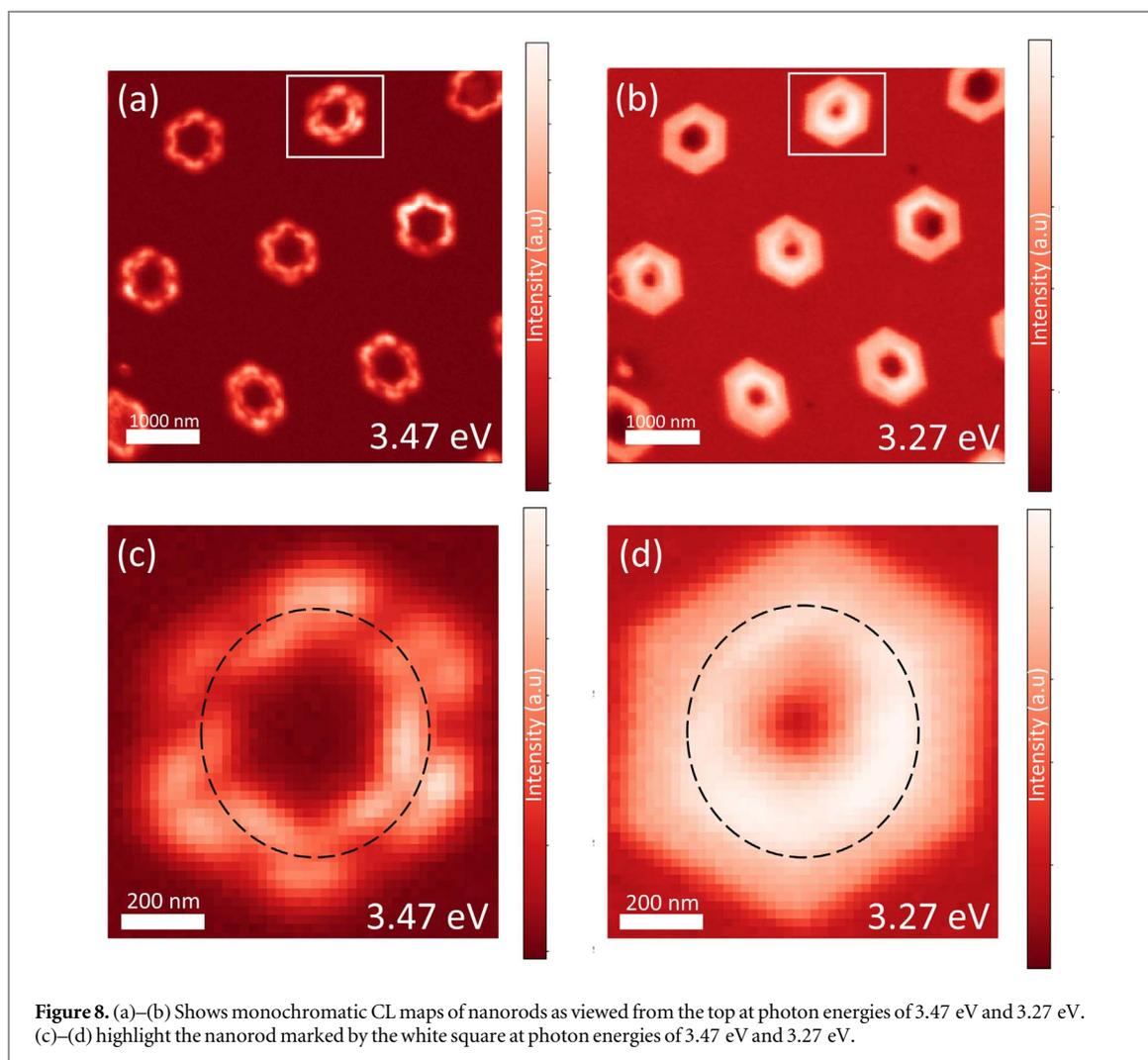
**Figure 8.** (a)–(b) Shows monochromatic CL maps of nanorods as viewed from the top at photon energies of 3.47 eV and 3.27 eV. (c)–(d) highlight the nanorod marked by the white square at photon energies of 3.47 eV and 3.27 eV.
