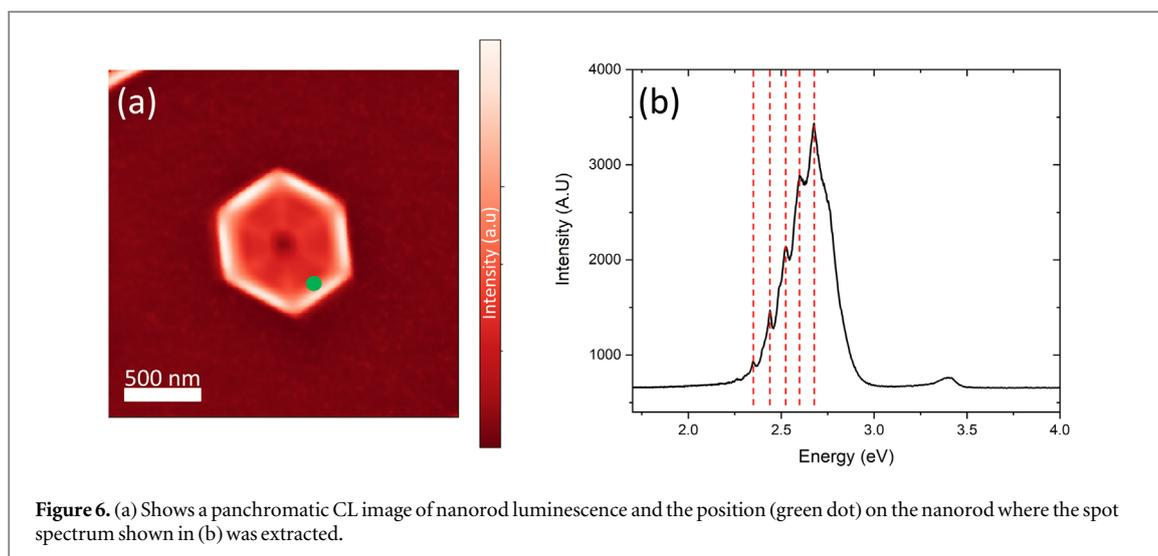
**Figure 6.** (a) Shows a panchromatic CL image of nanorod luminescence and the position (green dot) on the nanorod where the spot spectrum shown in (b) was extracted.
