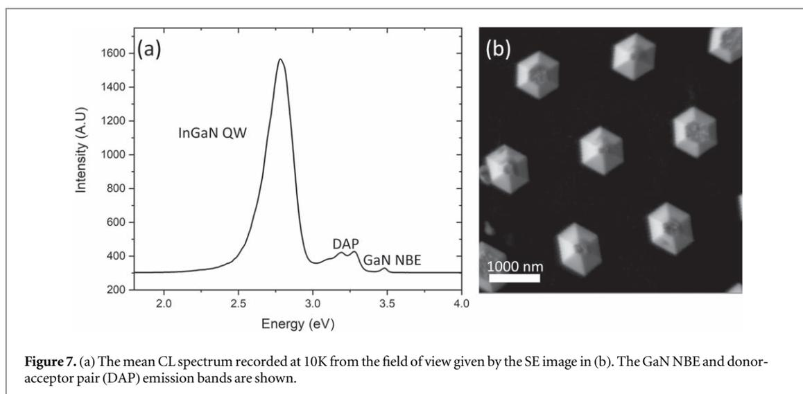
**Figure 7.** (a) The mean CL spectrum recorded at 10K from the field of view given by the SE image in (b). The GaN NBE and donor-acceptor pair (DAP) emission bands are shown.
