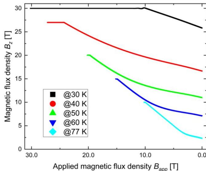
**Figure 2.** Magnetic flux density during the field-cooled magnetization (FCM) of an Ag-containing Gd-Ba-Cu-O bulk of radius  $R = 12.5$  mm and height  $D = 25$  mm at the centre reinforced by a ring of thickness  $r = 3$  mm for different temperatures.
