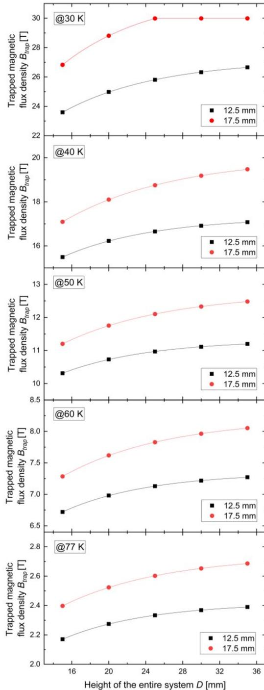
**Figure 13:** Trapped field at the end of the FCM process of an Ag-containing Gd-Ba-Cu-O bulk of radii  $R = [12.5 \text{ mm}; 17.5 \text{ mm}]$  reinforced by a ring of thickness  $r = 3 \text{ mm}$  for several heights  $D$  (15 mm – 35 mm), as well as different temperatures (30 K – 77 K).
