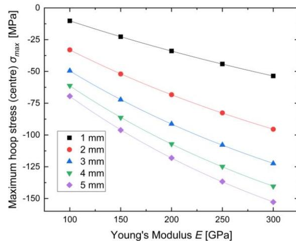
**Figure 16:** Maximum hoop stress at the centre of an Ag-containing Gd-Ba-Cu-O bulk of radius  $R = 12.5 \text{ mm}$  and height  $D = 25 \text{ mm}$  reinforced by a ring of thickness  $r$  (0 mm – 5 mm) and Poisson's ratio  $\nu = 0.3$  for several values of Young's modulus  $E$  (100 GPa – 300 GPa) of the ring material at 60 K.
