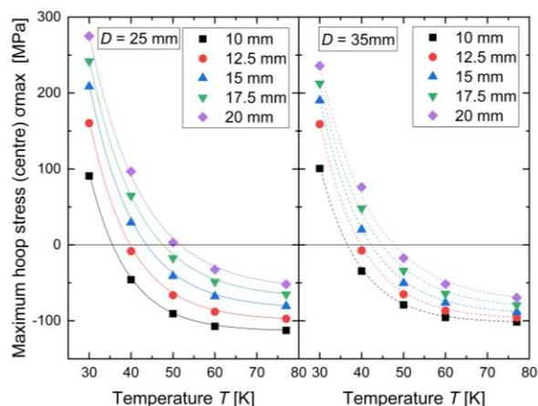
**Figure 7.** Maximum hoop stress at the centre of Ag-containing Gd-Ba-Cu-O bulk of heights  $D = [25 \text{ mm}; 35 \text{ mm}]$  reinforced by a ring of thickness  $r = 3 \text{ mm}$  for radii  $R$  (10 mm – 20 mm), as well as different temperatures (30 K - 77 K).
