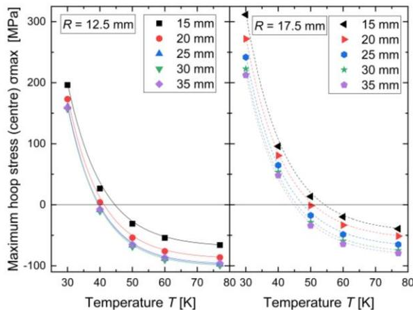
**Figure 5.** Maximum hoop stress in the centre of an Ag-containing Gd-Ba-Cu-O bulk of radius  $R = [12.5 \text{ mm}; 17.5 \text{ mm}]$  reinforced by a ring of thickness  $r = 3 \text{ mm}$  for several values of height  $D$  (15 mm – 35 mm) as well as different temperatures (30 K – 77 K).
