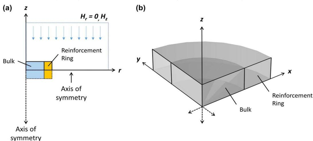
**Figure 1.** (a) Setup of a 2D axisymmetric numerical model of a (RE)BCO bulk with a reinforcement ring and an applied magnetic field in the  $z$ -direction in the  $r$ - $z$ - $\phi$  cylindrical coordinate system, as evaluated in [4]. (b) The equivalent 3D model [4]. © IOP Publishing. Reproduced by permission of IOP Publishing from [4]. All rights reserved.
