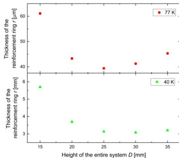
**Figure 12.** Minimum thickness of the ring reinforcement  $r$  required to provide compression at the centre of an Ag-containing Gd-Ba-Cu-O bulk of radius  $R = 12.5$  mm for the entire magnetisation process for several heights  $D$  (15 mm – 35 mm), as well as different temperatures  $T = [40$  K;  $77$  K].
