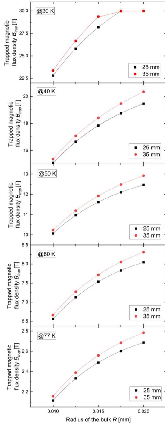
**Figure 14:** Trapped field at the end of the FCM process of an Ag-containing Gd-Ba-Cu-O bulk of heights  $D = [25 \text{ mm}; 35 \text{ mm}]$  reinforced by a ring of thickness  $r = 3 \text{ mm}$  for several radii  $R$  (15 mm – 35 mm), as well as different temperatures (30 K – 77 K).
