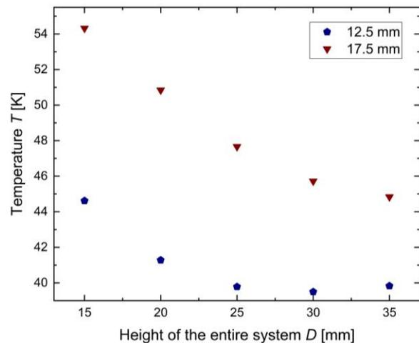
**Figure 6.** Minimum operating temperature, such that the centre of the Ag-containing Gd-Ba-Cu-O bulk of radius  $R = [12.5 \text{ mm}; 17.5 \text{ mm}]$  reinforced by a ring of thickness  $r = 3 \text{ mm}$  remains in a compressive state during the entire magnetization process for several values of height  $D$  (15 mm – 35 mm).
