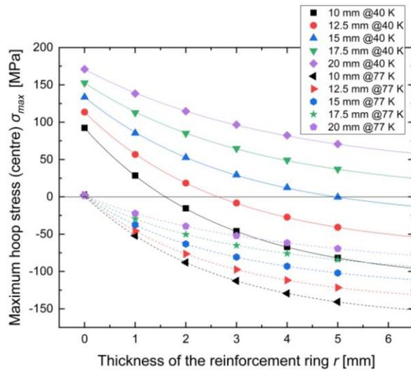
**Figure 9.** Maximum hoop stress at the centre of an Ag-containing Gd-Ba-Cu-O bulk with of height  $D = 25$  mm reinforced by a ring of thicknesses  $r$  (0 mm – 5 mm) for several radii  $R$  (10 mm – 20 mm), as well as different temperatures  $T = [40$  K;  $77$  K].
