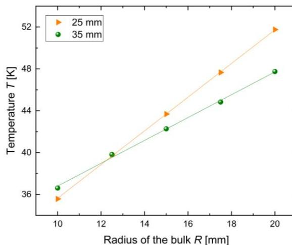
**Figure 8.** Minimum possible temperature, such that the centre of the Ag-containing Gd-Ba-Cu-O bulk of a radii  $R$  (10 mm – 20 mm) reinforced by a ring of thickness  $r = 3 \text{ mm}$  remains in a compressive state during the entire magnetization process for two heights  $D = [25 \text{ mm}; 35 \text{ mm}]$ .
