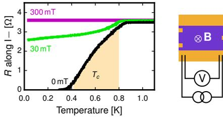
**Figure S4.** Superconducting behaviour in the I $-$  ohmic contact (left), showing the suppression of  $T_c$  when a magnetic field  $\mathbf{B}$  is applied perpendicular to the 2DEG. These resistance measurements along the top of the contact were performed on the 4 mm $\times$ 4 mm device on a separate cool-down using a different wire bond configuration (right).
