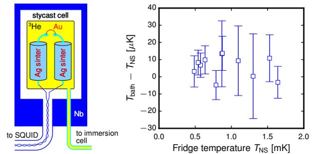
**Figure S5.** Thermalisation of  $^3\text{He}$ . In the plastic cell  $T_{\text{bath}}$  was measured directly using a  $^3\text{He}$  noise thermometer appendix (left). It agrees with the noise thermometer monitoring the nuclear stage temperature  $T_{\text{NS}}$  to within 20  $\mu\text{K}$  (right). Error bars represent s.e.m.
