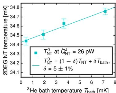
**Figure S6.** The fraction  $\delta$  of the 2DEG NT resistance sitting at the  $^3\text{He}$  bath temperature  $T_{\text{bath}}$ . Here we present the raw 2DEG NT readings  $T_{\text{NT}}^0$  versus  $T_{\text{bath}}$  when high power is applied to the NT heater, such that the temperature  $T_{\text{NT}}$  of the NT gold wire is independent of  $T_{\text{bath}}$ . A fit based on Eq. (S1) allows us to determine  $\delta$ . Error bars represent s.d.
