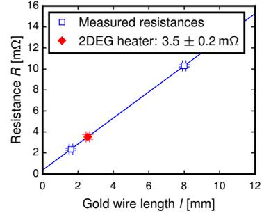
**Figure S2.** The resistance of the 2DEG NT heater is inferred from its length from  $R(l)$  measurements on similar wires of different lengths, all connected with wedge-bonded superconducting aluminium wires. The non-zero intercept in the  $R = a + bl$  fit is attributed to the gold-aluminium contact resistance. Error bars represent s.d.
