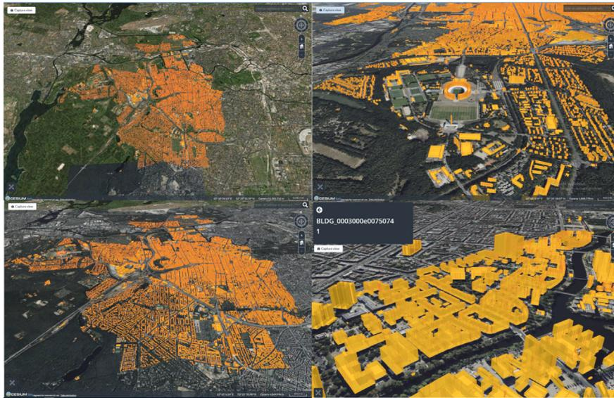
Fig. 7. Different views of a Charlottenburg-Wilmersdorf dataset visualised using KML files exported by the *CityExportAgent* from the Semantic 3D City Database of the Cities Knowledge Graph. The KML files contain the city model in LOD2 in extruded footprint display form.
