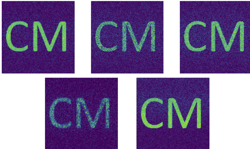
Fig. 3. Simulated replay fields retrieved from target image CM; Top Left: Cimmino FFT (CM FFT); Top Middle: Cimmino Full (CM Full); Top Right: Cimmino Eye (CM Eye); Bottom Left: Gerchberg-Saxton (GS); Bottom Right: Kaczmarz (KZ)
