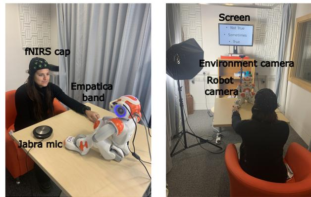
Fig. 1. Figures depicting the experimental setup that includes: the Nao robot, fNIRS cap, Empatica wrist band, Jabra mic, the Nao robot, the external camera, and the screen. The left figure depicts the lateral view of the setup where the participant is seated in front of the Nao robot, the right figure shows the perspective of the same setup from the back. Actual pictures from the CHRI sessions have not been used in order to protect the privacy of the child.
