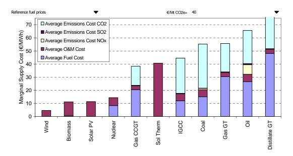
Figure 5 Change of marginal generation costs after introduction of CO2 emission certificates.<sup>110</sup>
