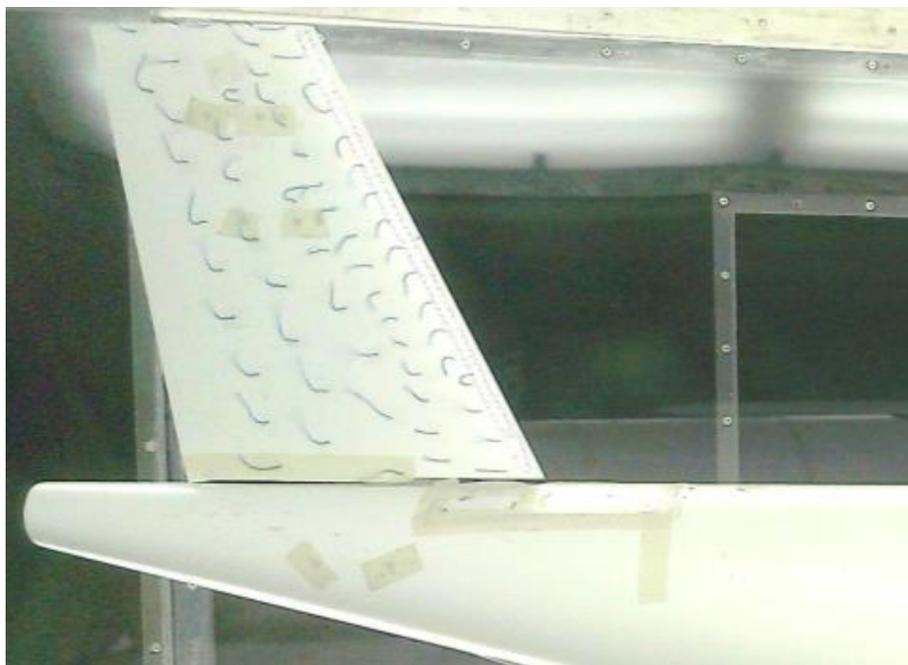
Fig. 2.8 Flow visualization over a VTP at  $\beta = 20^\circ$  and  $\delta_r = 0^\circ$  [76].
