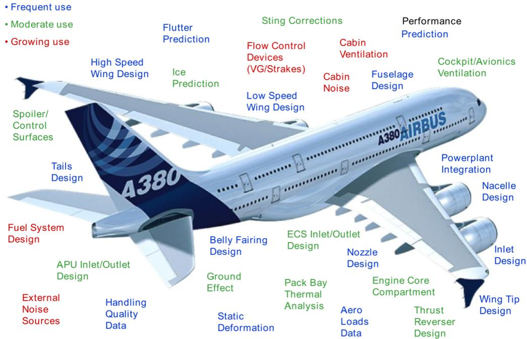
Fig. 2.10 Use of CFD for the aerodynamic design of an Airbus A380 aircraft [2].
