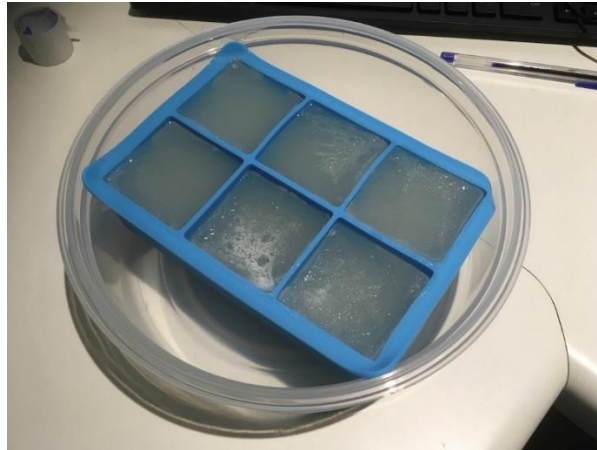
SI Figure 2: Six compartment phantom in silicone ice cube tray with six different concentrations of creatine (0, 5, 10, 20, 40, and 80 mmol/L). Each compartment is roughly 4.8 \times 4.8 \times 4.8 \text{ cm}^3 .
