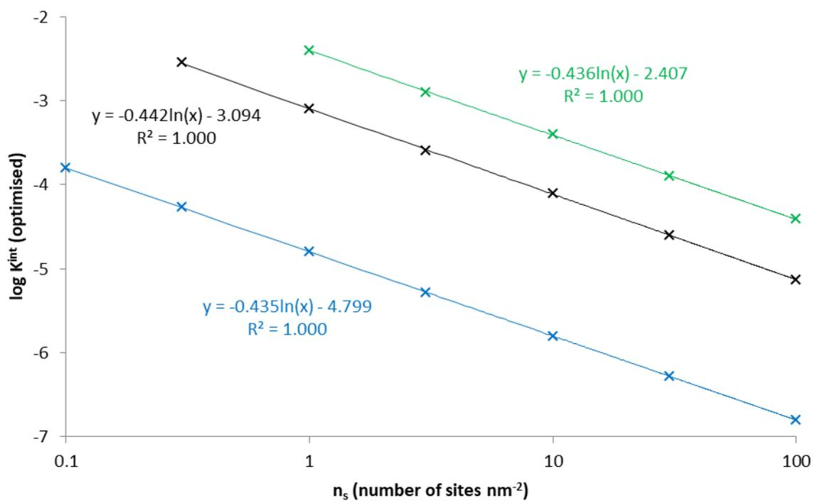
Figure S5: A graph showing the different site densities ( $n_s$ ) used to fit the experimental salt-solution titration data with numerical modelling for Na (blue), Mg (black) or Ca (green) and ( $\log_{10}$  of) the equilibrium constant ( $K^{\text{int}}$ ) that provides the best fit in each case. The linear relationships observed in this log-log plot lead to Equation 10.
