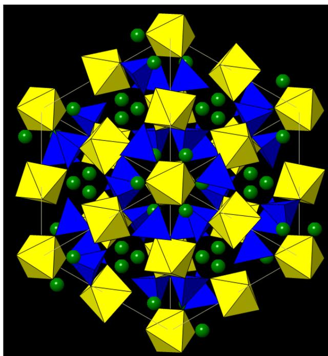
Figure S1: A unit cell of the almandine garnet crystal structure in polyhedral representation. Yellow octahedra are  $\{\text{AlO}_6\}$  units, and blue tetrahedra are  $\{\text{SiO}_4\}$  units. Green atoms are Fe, residing in large 'voids' within the octahedral-tetrahedral framework.
