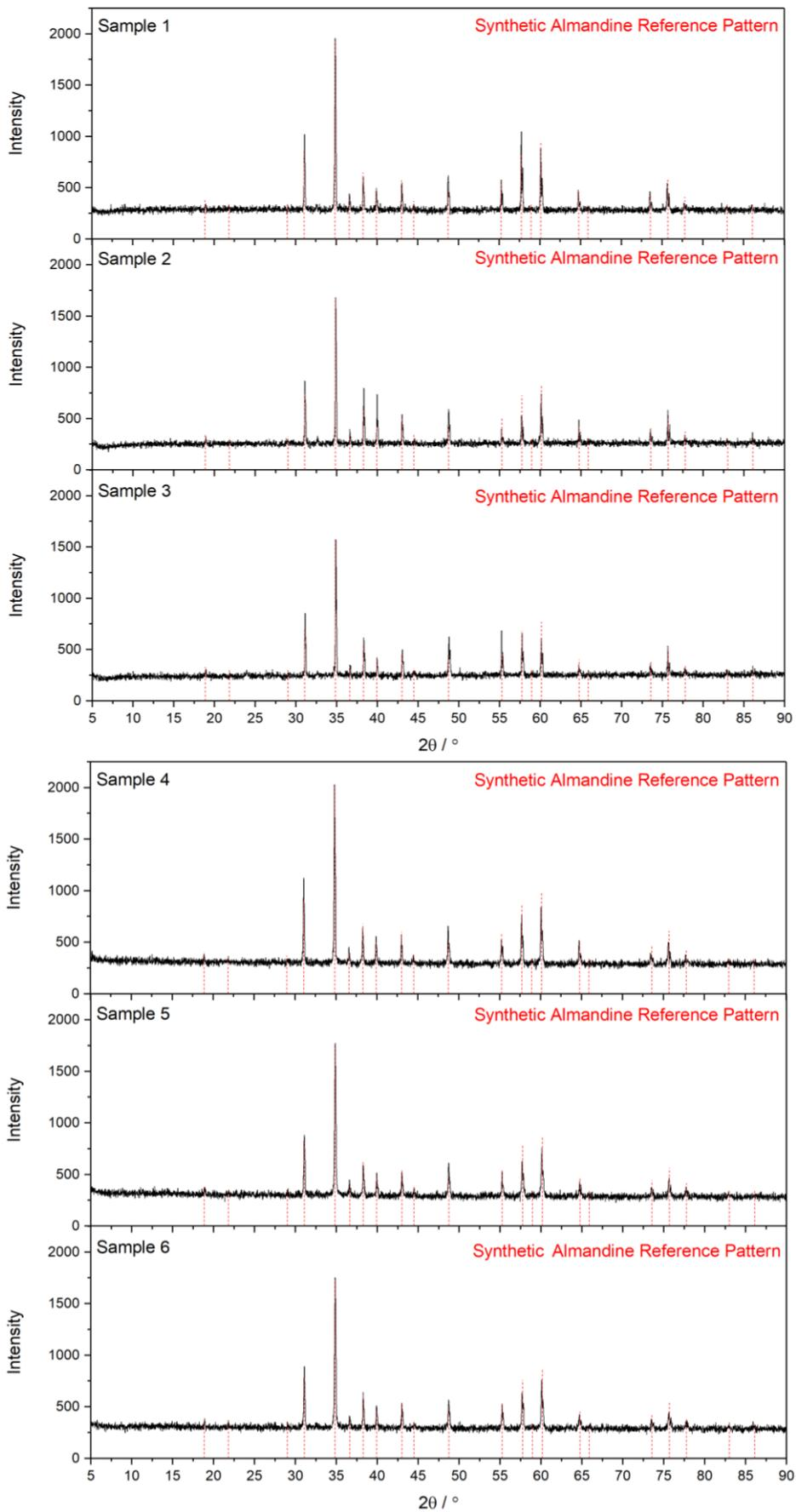
**Figure S2: Powder X-ray diffraction data of almandine garnet before (samples 1-3) and after (samples 4-6) acid washing. The powders were tumbled for one week in 0.1 M HCl (samples 1 and 4), ultrapure water (samples 2 and 5) or 0.1 M NaOH (samples 3 and 6); all show good agreement with the reference**
