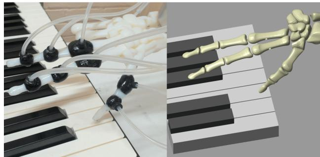
Fig. 1. Anthropomorphic three-fingered robot hand with variable stiffness joints and its simulated replication.
