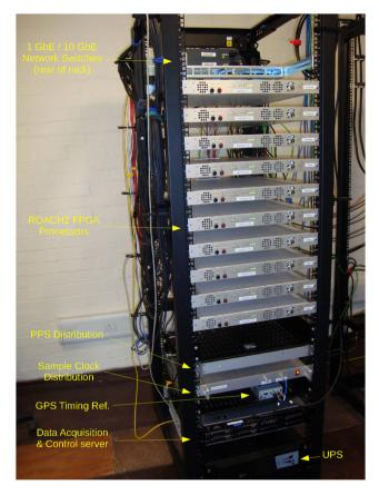
Figure 4. The digital correlator rack for the 10-antenna AMI SA.
