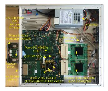
**Figure 3.** The CASPER ROACH2 platform on which the AMI digital correlator is implemented. Here, the board is shown with two 5 Gsps ADC daughter cards, a quad-SFP+ mezzanine card, and a Walsh switch interface hox
