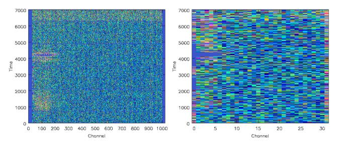
**Figure 8.** An illustration of RFI removal from the LA observation shown in Fig. 7. The left-hand side shows the effect of a  $5\sigma$  flagging step using the CASA 'rflag' algorithm; the bright, narrow-band signals have been removed as well as some of the wider-band signals. On the right, we have binned in frequency down to 32 channels and made another  $5\sigma$  cut, which removes most of the remaining wider-band signals.
