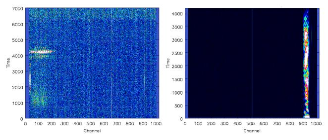
Figure 7. 'Waterfall' plots of a low-declination ( $\approx 0^{\circ}$ ) field observed with the LA (SA) on the left (right), showing time against channel for the lower (upper) half of the bandwidth on a single baseline. The RFI can be clearly seen as bright signals localized in frequency and time and is easily removed using automated algorithms such as 'rflag' in CASA; see Fig. 8.
