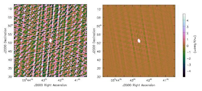
**Figure 9.** An LA observation of the bright, unresolved source 3C147 using the old (new) correlator on the left (right). The colour scales are the same, and have been truncated to show the systematic residuals around the source. These are at most 9.3 (1.1) mJy beam<sup>-1</sup>, giving a dynamic range of 260 (2300).
