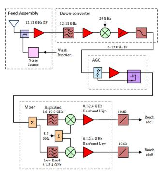
**Figure 1.** The AMI RF and IF system diagram. Isolators and attenuators used in the chain are not shown. The *Mixer* units in the system are newly developed as part of the correlator upgrade.
