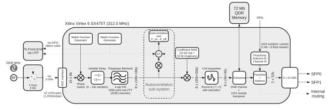
Figure 5. A schematic depiction of the AMI F-Engine firmware. Two such F-Engines are instantiated on each ROACH2 FPGA.
