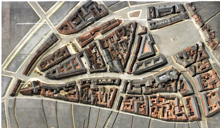
Figure 58: The so-called Great Breakthrough, a boulevard designed by the architect and planner Fritz Beblo, combined radical infrastructural modernisation with a new attention to the urban context. Beblo's design weaves through the inner city, featuring gentle curves, carefully-framed views of historical monuments, and unexpected connections to the adjoining lanes. Model by Emile Maechling (1878-1964). Credit: Musées de Strasbourg.
