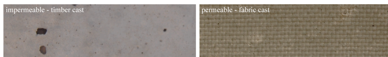
Figure 1 – Identical concrete cast in impermeable (left) and fabric (right) moulds.
