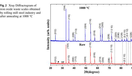
minor iron oxides components. In this case, the presence of those peaks indicate the complete oxidation of magnetite [15], as detected by the other techniques below.
