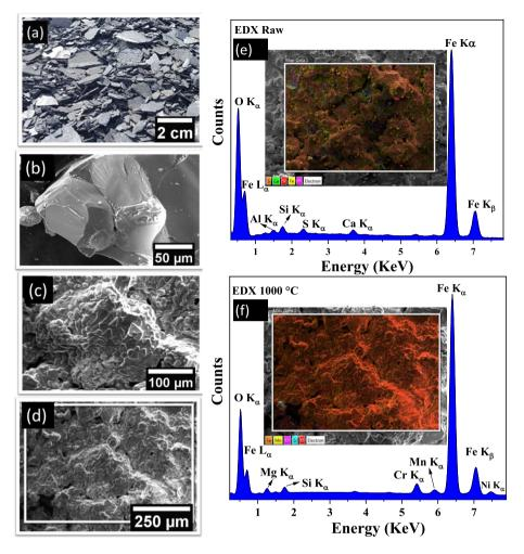
Fig. 1 SEM micrographs and EDX analysis of iron oxide waste scale obtained by rolling mill steel industry and after annealed at 1000 °C. **a**) and (**b**) micrographs of the collected scale samples and (**c**), (**d**) micrographs for the annealed sample at 1000 °C. (**e**) and (**f**) EDX for raw sample and after annealing at 1000 °C
