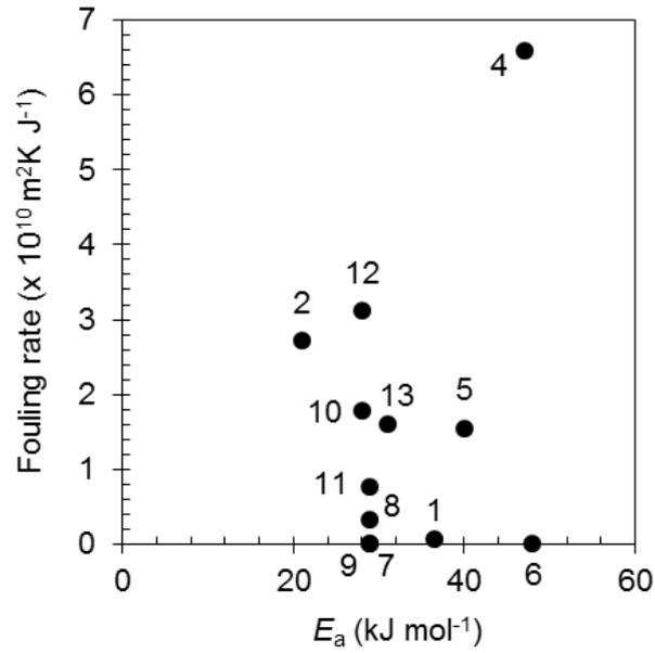
Fig. 4 Fouling rate predicted for benchmark conditions (velocity  $2 \text{ m s}^{-1}$ ,  $Re = 17100$ ,  $Pr = 10$ ,  $T_f = 503 \text{ K}$ ,  $\tau_w = 7.2 \text{ Pa}$ ) using the parameters reported in Table 1 (labels given in Table 1). Equation [A] predicted negative values for 6, 7 and 9 so these are plotted as zero.
