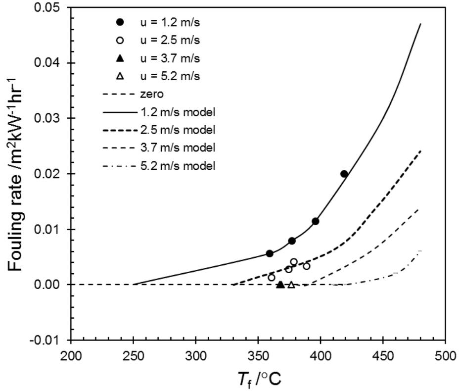
Fig. 2 The Ebert-Panchal model, Equation (1), fitted to Scarborough *et al.*'s data [6], reproduced from Ebert and Panchal [11]. Loci plotted for parameters  $a_1 = 30.2 \times 10^6$   $\text{K m}^2/\text{kW h}$ ;  $b_1 = -0.88$ ,  $c_1 = 1.45 \times 10^{-4}$   $\text{m}^2 \text{K m}^2/\text{kW Pa h}$  and  $E_a = 68$   $\text{kJ/mol}$ .
