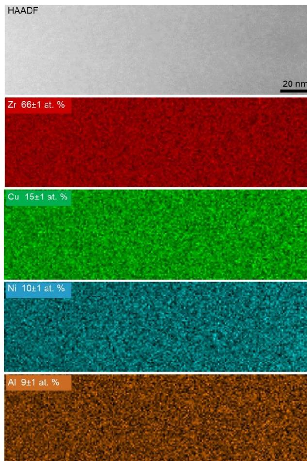
**Extended Data Fig. 4 | TEM of the central region of a rejuvenated  $\text{Zr}_{64.13}\text{Cu}_{15.75}\text{Ni}_{10.12}\text{Al}_{10}$  MG sample.** The high-angle annular dark-field (HAADF) image and the EDX maps show the sample to be structurally and chemically homogeneous. The measured elemental contents are close to the nominal values. at. %, atomic percentage.
