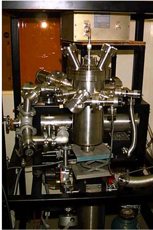
Figure 3.11: The silica deposition system.
