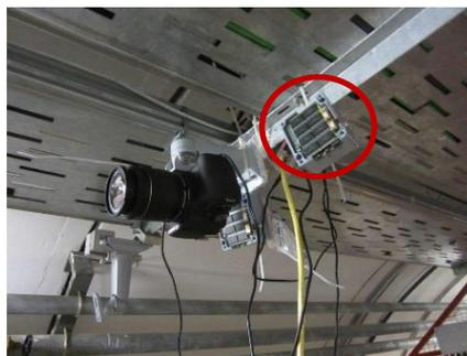
**Figure 4.1.** Radiation dosimeters installed on the TT10 tunnel crown (Di Murro et al. 2019).
