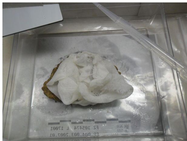
Figure 5 Wall plaster fragments, lifted with cyclododecane on cotton gauze, during impregnation with an ethyl silicate. Photo: ASCB.
