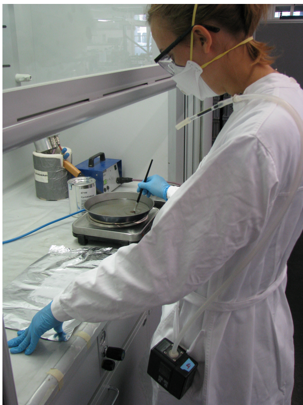
Figure 7 Workplace exposure measurements for molten cyclododecane applied by brush under an operative exhaust hood. Photo: ASCB.
