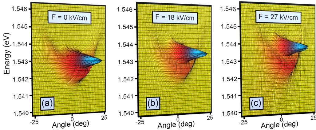
FIG. 2. Angle-dependent polariton far-field emission under nonresonant continuous wave excitation recorded on the logarithmic scale. A gradual blueshift of polariton condensate energy is observed when the electric field is applied: (a) zero bias, (b) 15 kV/cm, and (c) 24 kV/cm. Superimposed weak emission arising from noncondensed low-excitation density areas of the sample surrounding the central spot shows a similar energy blueshift.
