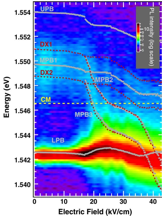
FIG. 4. Normal incidence PL emission with varying applied bias. Bare uncoupled exciton branches are shown by dotted line. LPB, MPB, and UPB polariton emission peaks are fitted by using the coupled harmonic oscillator model using the exciton energy and linewidths measured from PL measurements on bare QWs. A LPB energy blueshift occurs due to Rabi-splitting reduction caused by free-carrier-induced broadening of the low-lying exciton branch at the onset of LO-phonon-assisted tunneling.
