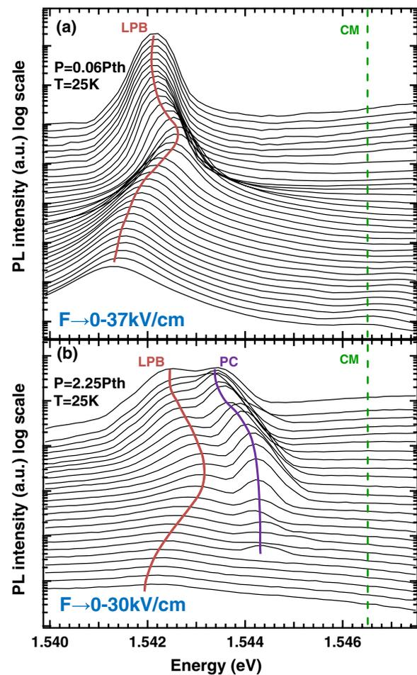
FIG. 3. PL spectra recorded at normal incidence to the sample plane for an increasing electric field (a) below and (b) above the condensation threshold, respectively. Low-density lower polariton branch emissions arising from the outer part of excitation spot are marked with (LPB), whereas bias-dependent condensate energy is marked by a polariton condensate (PC) line.
