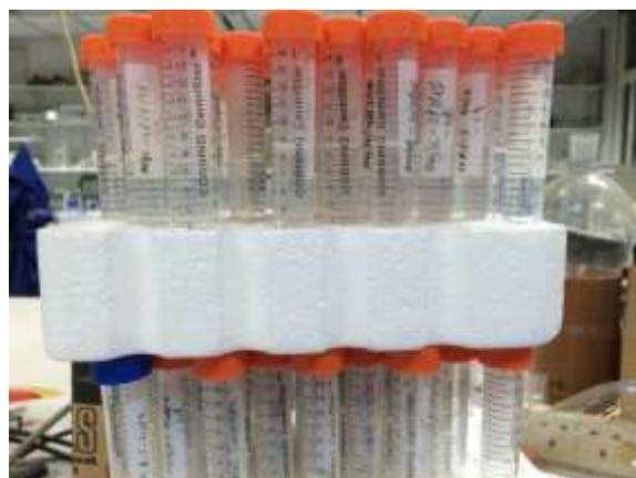
(c): Typical acidified samples for ICP testing
