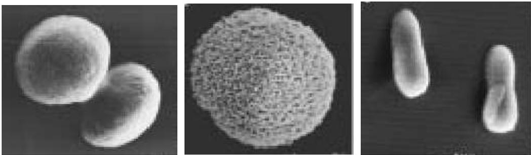
(a): The SEM of precipitates grown in the presence of 4:1 Mg/Ca solution from left to right-- Magnesian calcite spherulite with typical dumbbell morphology; Polycrystalline aragonitic spherulite, with the needle shaped morphology of single crystallites with magnesian calcite core(see next figure); Elongated magnesian calcite particles, such particles contain the highest magnesium contents (Raz et al., 2000)
