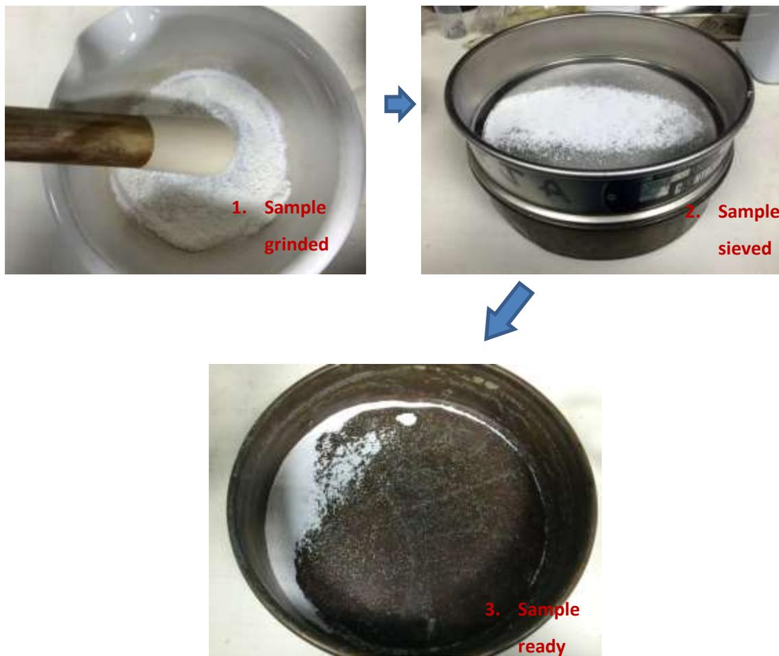
(c): The preparation of oxides for a reactivity test
