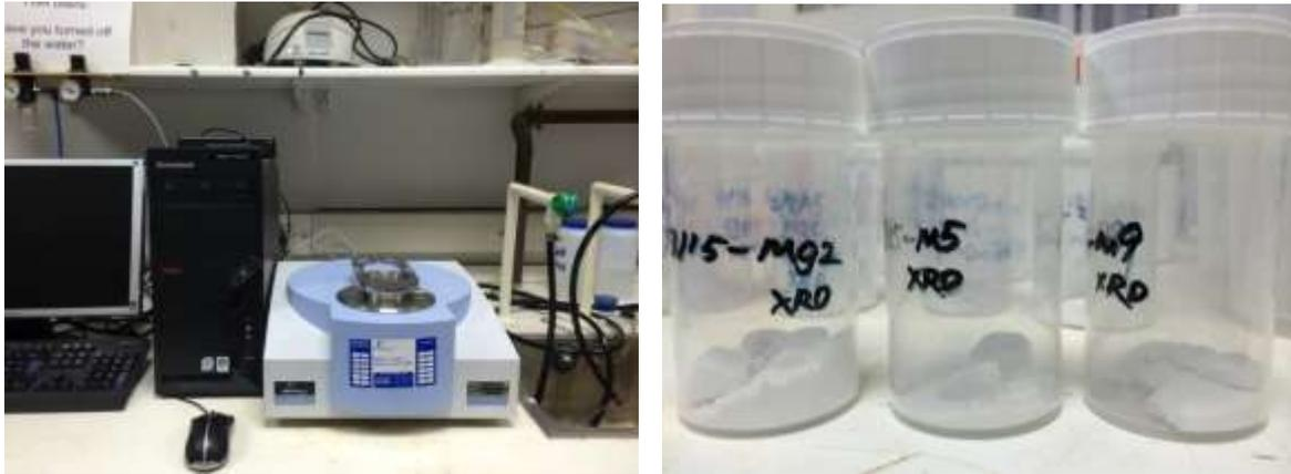
Figure 3. 9: Perkin Elmer STA 6000 TGA (left); Samples used for both XRD and TGA (right)
