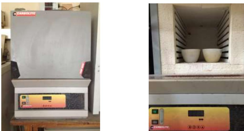
(b): Furnace used in calcinaing HMCs
