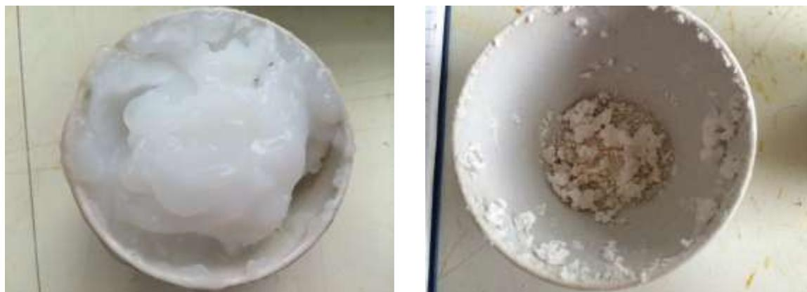
**Figure 3. 5: Carbonates with colloidal property before calcination (left), oxides with aggregated chunks after calcination (right).**
