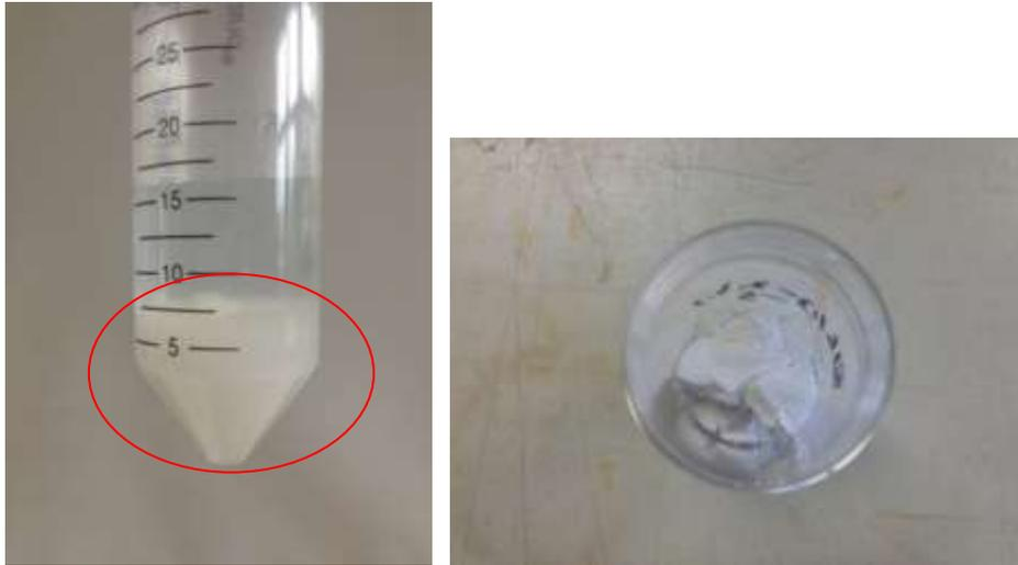
(a): Precipitates obtained from pH =8.75 after 30min bench reaction of SI.I
