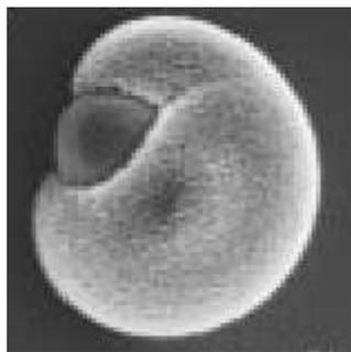
(b): A mixed particle with a core of polycrystalline magnesian calcite and an outer shell of polycrystalline aragonite (Raz et al., 2000)
